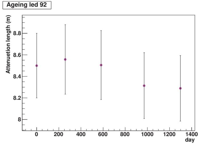
Figure 86: Evolution of the attenuation length with time for LED 92. The four  $\lambda_i$  obtained from the fits, and the  $\lambda_0$ , are plotted as a function of the elapsed days, starting from  $t_0$ .
