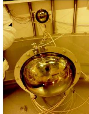
(c) A PMT with two fibres attached.
