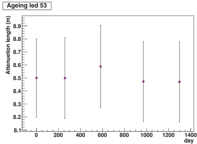
Figure 87: Evolution of the attenuation length with time for LED 53. The four  $\lambda_i$  obtained from the fits, and the  $\lambda_0$ , are plotted as a function of the elapsed days, starting from  $t_0$ .
