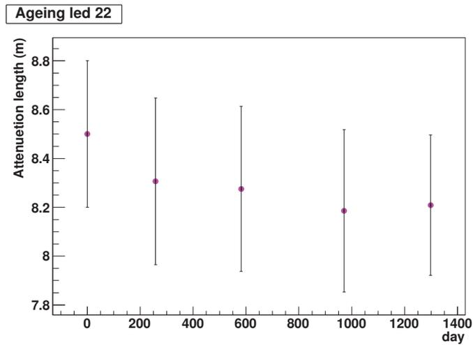
Figure 89: Evolution of the attenuation length with time for LED 22. The four  $\lambda_i$  obtained from the fits, and the  $\lambda_0$ , are plotted as a function of the elapsed days, starting from  $t_0$ .
