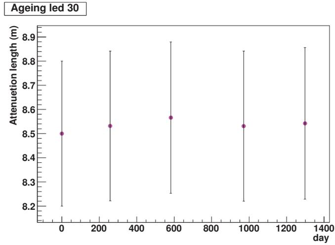
Figure 88: Evolution of the attenuation length with time for LED 30. The four  $\lambda_i$  obtained from the fits, and the  $\lambda_0$ , are plotted as a function of the elapsed days, starting from  $t_0$ .
