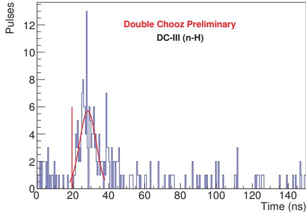
Figure 69: Example of a shifted PS. The red curve represents the Gaussian fit around the maximum to compute the shift. The shift value of 19 ns is represented by the vertical red line ( $1.8 \sigma$  on the left with respect to the fitted mean). The pulses on the left side of the vertical red line are interpreted as the result of a low energy proton recoil.
