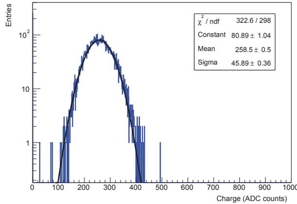
Figure 81: Charge collected by the reference PMT during a calibration run with the LED number 53 of the IVLI system. A gaussian fit on the distribution is represented by the black solid line.
