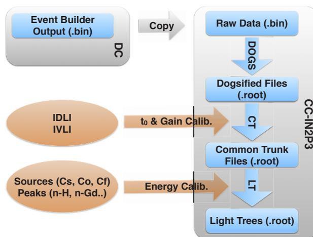
Figure 24: Diagram showing the data processing of recorded events in Double Chooz. Data processing steps are featured in blue and the operation platforms in grey, while calibration inputs are represented in orange.
