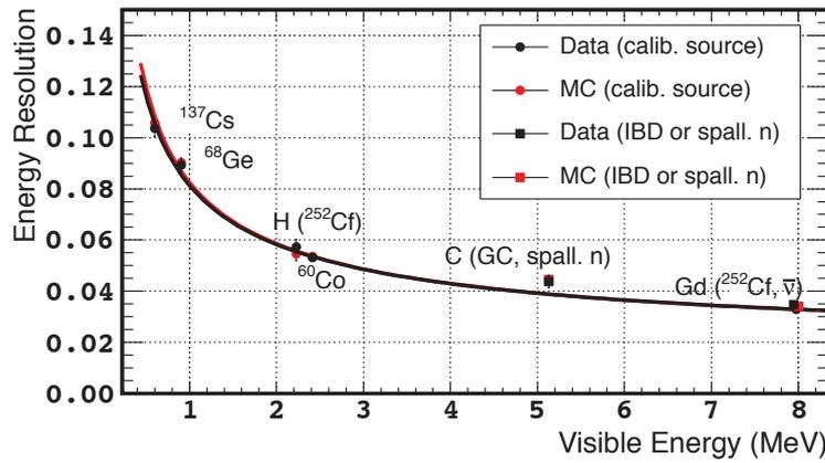
Figure 26: Data-MC comparison of the visible energy resolution from [160]. The values measured with different energy peaks are fitted with the fit function of equation 59.
