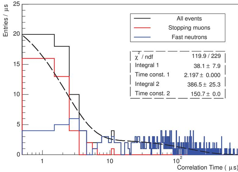
Figure 60:  $\Delta t$  of an OV sample of DC-III (n-H), separated into total events (black), stopping muons (red) and fast neutrons (blue) according to the PS log-likelihood analysis. The total distribution is fitted with a combination of two exponentials, with fixed time constants and integrals left free.
