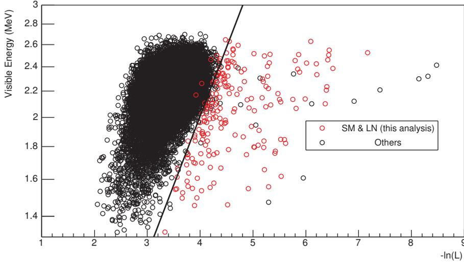
Figure 62: Energy of the delayed events, as a function of FuncV ( $-\ln(L)$ ), of an enriched IBD sample obtained by applying full candidate selection with the exclusion of the FuncV cut, which is represented by the black line. Events selected with the PS log-likelihood analysis are featured in red.
