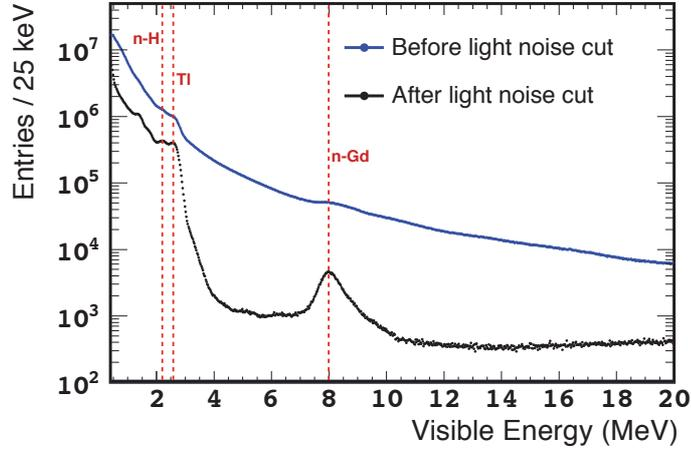
Figure 28: Visible energy of single events before (blue) and after (black) the light noise cuts are applied. Energy peaks for neutron capture on Gd and H, as well as  $^{208}\text{Tl}$   $\gamma$  decay, are highlighted (red dashed lines). From [160].
