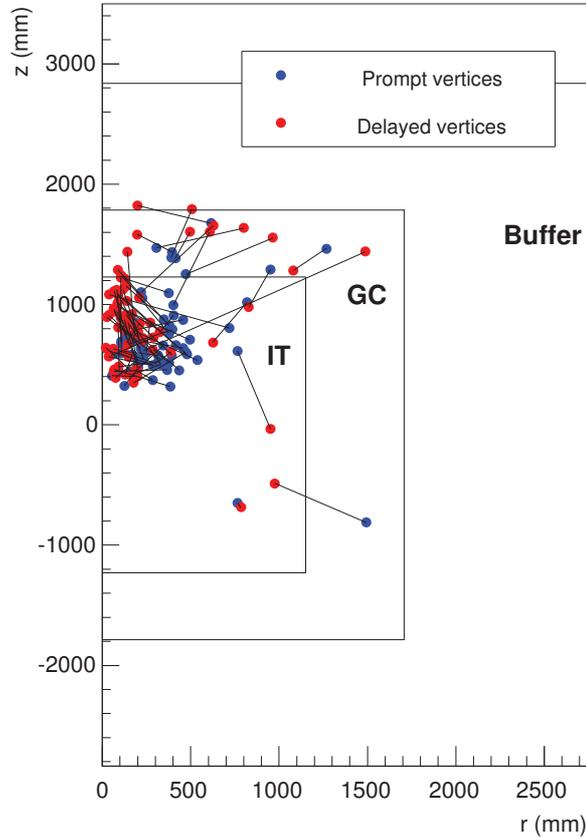
Figure 42: Detector schematic section showing the vertex distribution of stopping muons (with a small component of fast neutrons) selected using the OV tag and the prompt-delayed correlation time ( $\Delta t < 10 \mu\text{s}$ ). The black lines represent the borders between the inner target (IT), the gamma catcher (GC) and the buffer. Every set of a blue and a red dot connected by a solid line represents the prompt and the delayed vertex position of the event.
