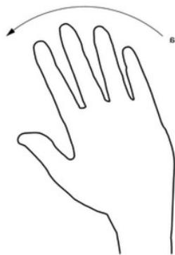
Figure V.9 Illustration: radial deviation (adapted from ISO 9241-400:2007)
