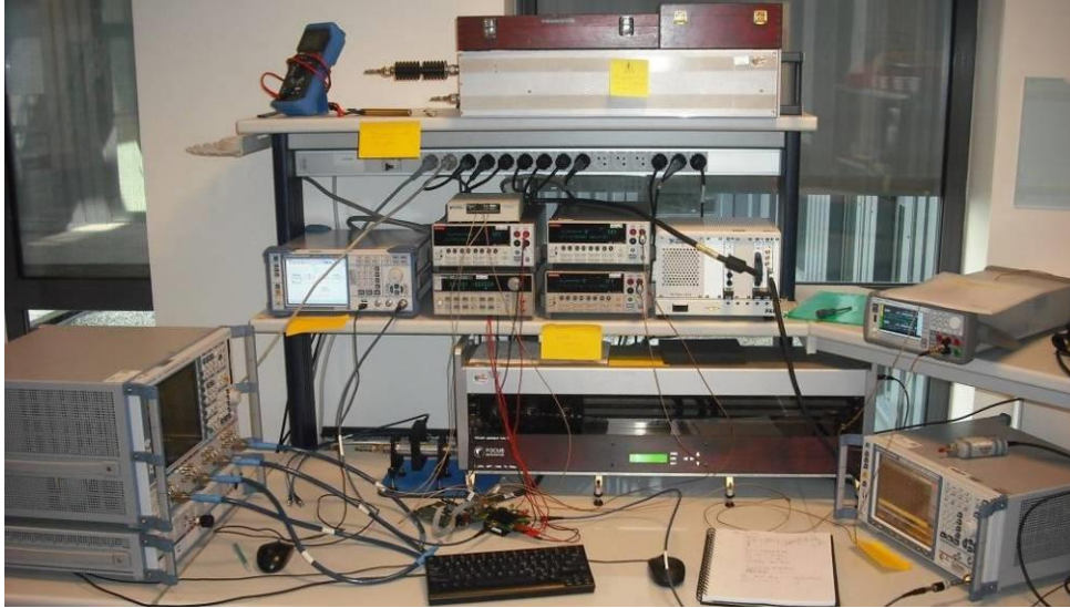
Figure 90: Photograph of the test bench for reconfigurable MMPA characterization
