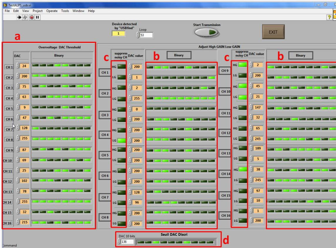
Figure 4.3: Labview interface(I). a) 8-bit words for overvoltage adjustment by per macro-pixel DAC 8-bit, b) 8-bit words for high/low gain adjustment via R-2R blocks, c) high/low gain noisy channel suppression ( $no\_CB$  bits), d) 10-bit word to the DAC 10-bit for discriminator threshold adjustment.
