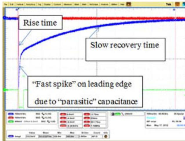
Figure 2.37: Output signal form of a SiPM ( $3.5 \times 3.5 \text{ mm}^2$ , 3600 cells, N-on-P structure)[63].
