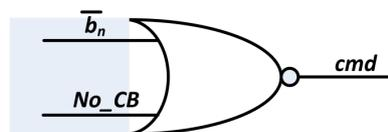
Figure 3.29: The generation of the command bit *cmd* for one multiplexer.
