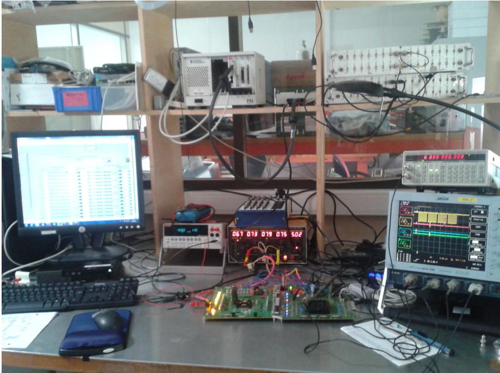
Figure 4.5: Test bench for chip electrical tests.
