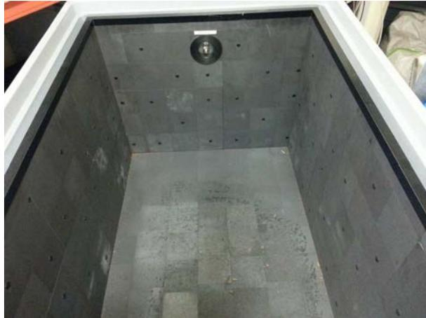
Figure 4.30: Photography of the anechoic container.
