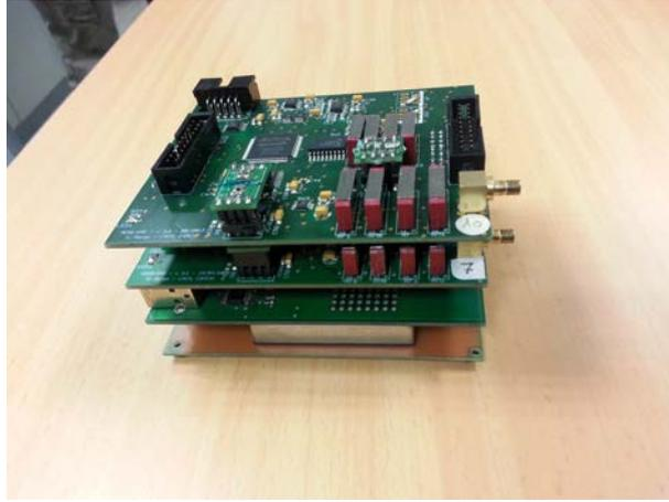
Figure 4.3: Capacitive sensor board.
