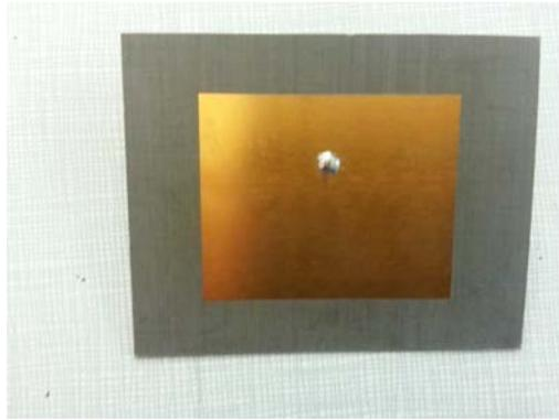
Figure 4.15: Microstrip patch antenna operating at 1 GHz,  $W = 91.3$  mm,  $L = 71.3$  mm.
