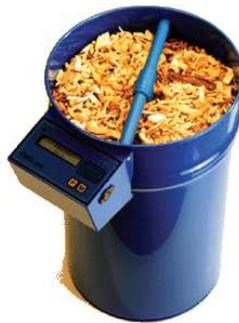
Figure 2.6: FMG 3000 - Moisture meter taken from [79].
