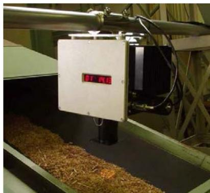
Figure 2.8: Optical Spectrometer Series KJT70, taken from [81].
