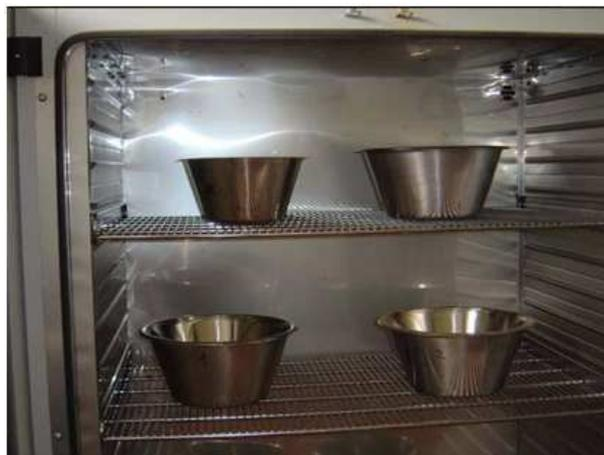
Figure 1.7: Samples of wood chips drying in an oven.
