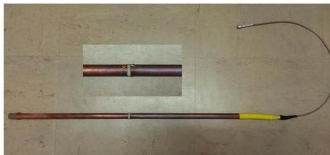
Figure 4.20: Photography of half-wave dipole fed in-line.
