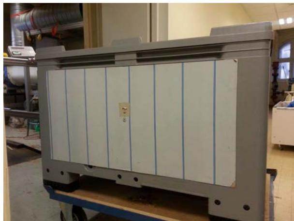
Figure 4.2: Capacitor implemented in a plastic container.
