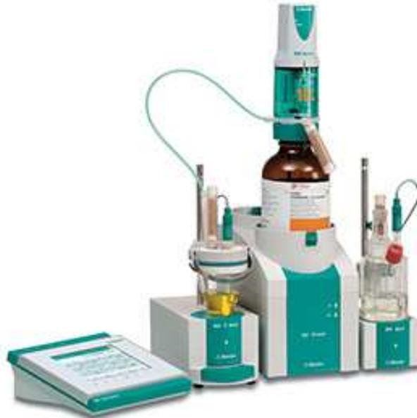
Figure 2.5: KF Titrator: Metrohm's instrument, taken from [66].
