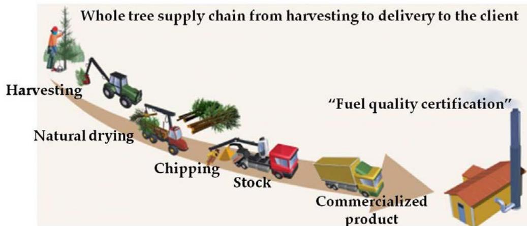
Figure 1.4: Production chain of wood chips, taken from [40].
