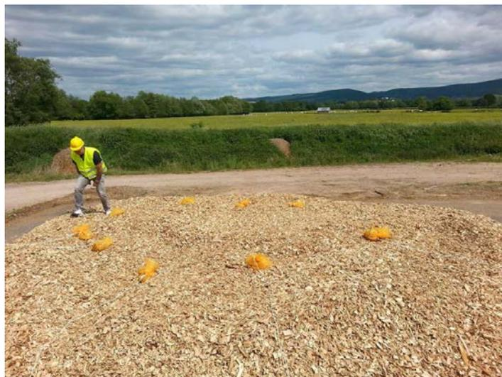
Figure 4.37: Samples of wood chips within the sampling piles.
