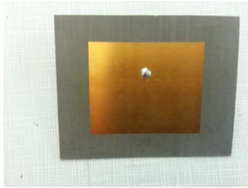
Figure 4.15: Microstrip patch antenna operating at 1 GHz, W = 91.3 mm, L = 71.3 mm.
