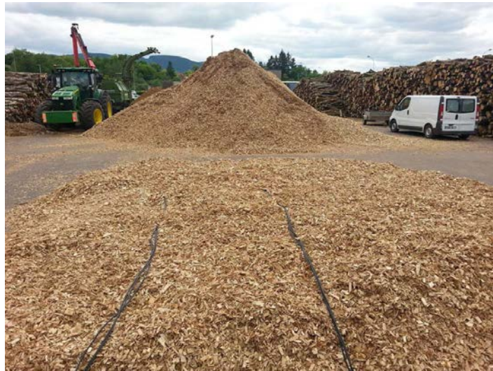
Figure 4.34: Installation of ropes of sensors while formation of the piles.
