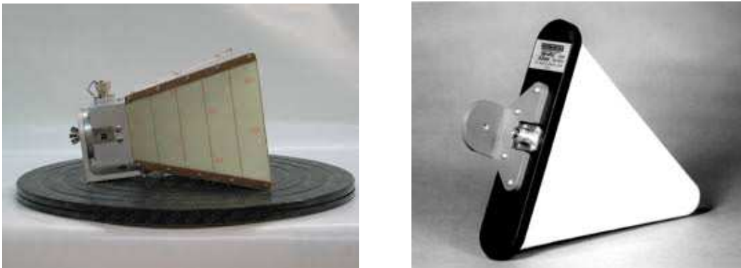
Figure 3.15: Transmission and reflection antennas.
