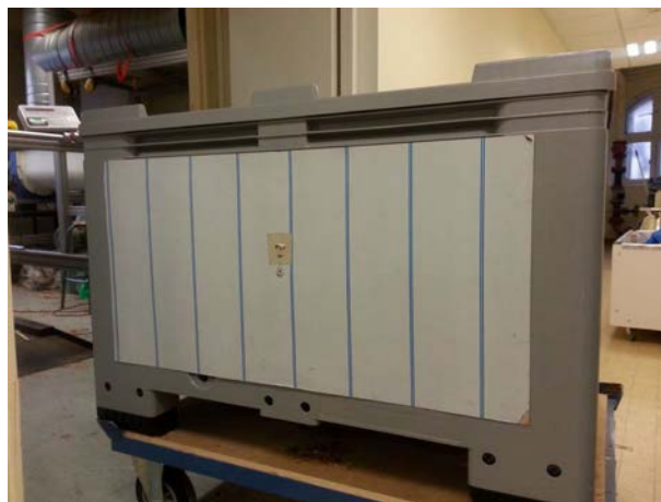
Figure 4.2: Capacitor implemented in a plastic container.
