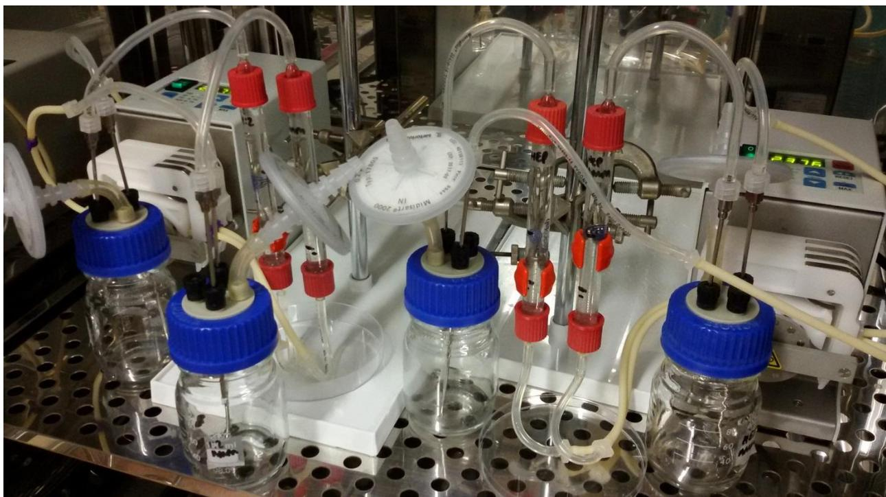
**Figure 9.** Multiple bioreactor-circuit set for independent control of distinct examined culture cases.
