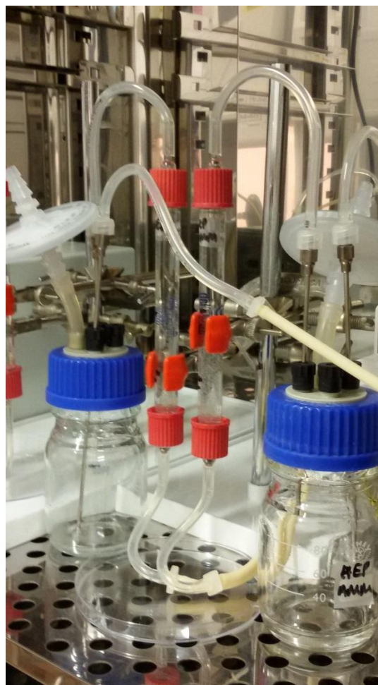
Figure 8. Small-scale glass fluidized bed bioreactors and complementary circuit accessories (medium filtered-gas-exchange reservoirs, connection tubes, and peristaltic pumps, on the back sides).
