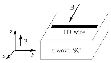
Figure 3.7: Scheme of the superconductor-semiconductor wire setup. 1D wire lies along the y axis, spin-orbit interaction u is along z axis and a magnetic field B is along x axis.
