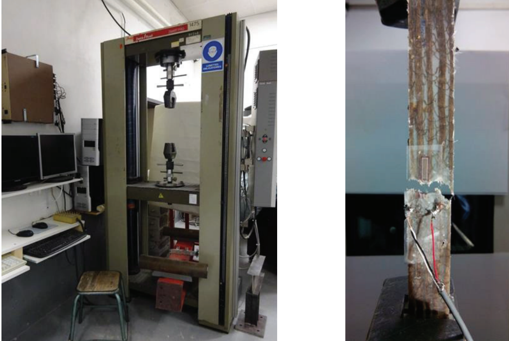
Figure 54: (a) Machine de traction universelle Zwick/1475, (b) Essai de traction sur composite.
