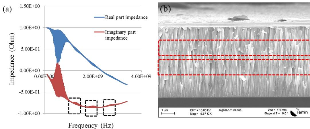
Figure 2.5.12 For the 5.7  $\mu\text{m}$  ZnO film on 100 nm Ti ground electrode, the interpreted impedance by VNA (a) and the cross-section of SEM of ZnO nanowires (b). In the dash box it was observed the multi-frequency and their incentive – the layering of ZnO.
