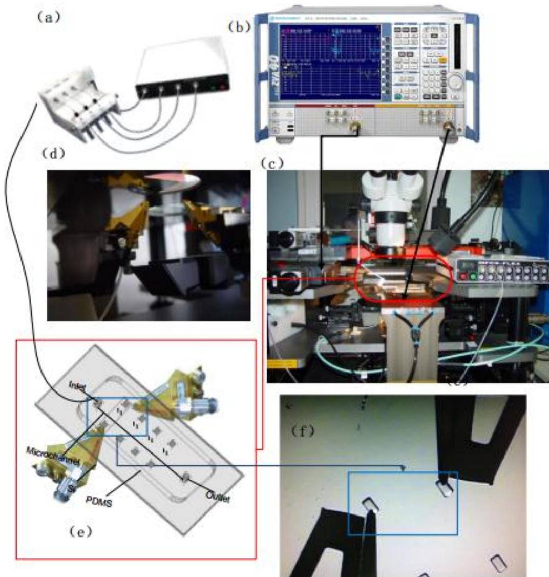
*Figure 3.1.4 Schematic diagrams of the whole setup for acoustic signals detection: (a) Pressure-driven flow controller for the microfluidic system, (b) The multi-channel signal generator, (c) Rhode&Scharwtz vector network for data analysis, (d) physical map of the positioned probes on the backside of the sample, (e) Sketch map of a package of the device, (f) observation of two probes contacted on ZnO transducers.*
