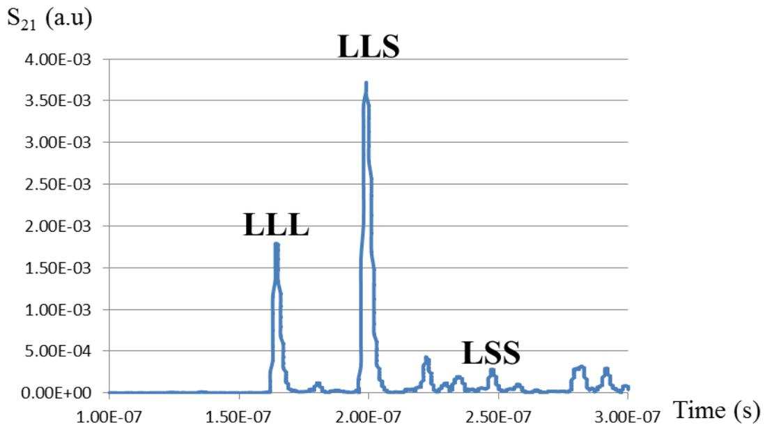
Figure 3.2.2  $S_{21}$  impulse response for sample 1 in time domain.
