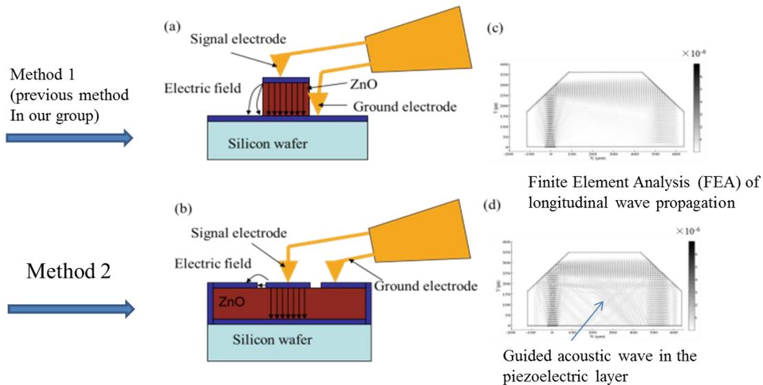
Figure 3.1.5 Scheme of the different configuration of ZnO transducer excitation and simulation for the amplitude of the longitudinal wave after reflected on  $45^\circ$  mirrors. (a) excitation on patterned ZnO, (b) excitation on ZnO full layer using patterned top electrodes, (c) simulation of longitudinal wave propagation from localized ZnO patterns, (d) simulation of longitudinal wave propagation from ZnO film on full layer but with localized top electrode patterns [9].
