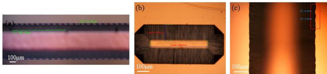
*Figure 2.2.10 (a) 3h etching for 70 μm depth mirror. SiO<sub>2</sub> layers with diffraction patterns are on the mirrors , (b) 7h etching for 160 μm depth mirror, (c) 9h etching for 210 μm depth mirror.*
