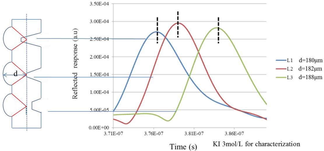
Figure 3.4.2  $S_{11}$  reflection coefficient parameters for KI solution in lens of different focal lengths. L1:  $d=180\mu\text{m}$ , time echo is 376 ns; L2:  $d=182\mu\text{m}$ , time echo is 379 ns; L3:  $d=188\mu\text{m}$ , time echo is 384 ns.  $d$ : distance between the reflector and the bottom of lens.
