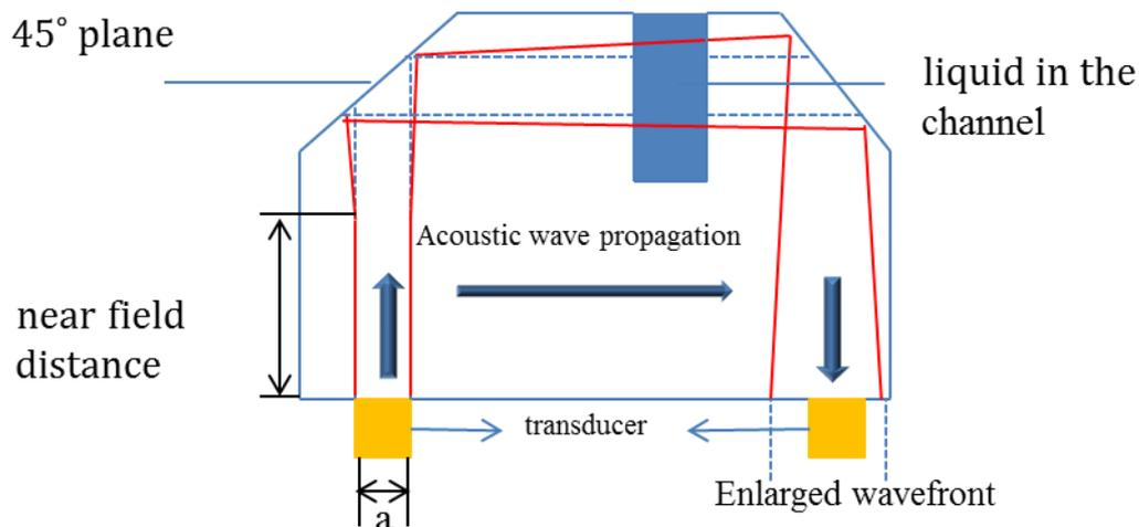
Figure 2.1.1 plane wave diffraction in our system. Near field distance  $d=214 \mu\text{m}$ , for a given transducer width  $a=120 \mu\text{m}$  and central frequency  $f=500 \text{ MHz}$ . The acoustic beams propagate mainly in the path of far field.
