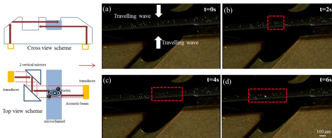
*Figure 3.6.2 Vortex induced by two travelling wave of 5dBm input power. Particles are  $9 \mu m$  in diameter. Strong acoustic streaming happened in dash box.*
