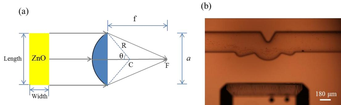
Figure 3.4.1 Scheme of the acoustic wave transmission through an acoustic lens. (a) structure chart of the cylindrical lens, (b) photo of the  $45^\circ$  mirror-lens system. The width of reflection wall is  $30\mu m$ .  $R$  is the radius of lens,  $\theta$  is the angle of aperture,  $a$  is the aperture,  $C$  is the center of the curvature and  $F$  is the focus. The length of transducer is the same with the aperture.
