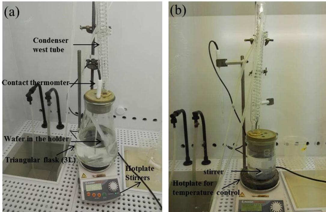
Figure 2.2.3 Schematic of the wet etching equipment (a) in 3L conical flask and thermomter control temperature and (b) in 1L beaker and hotplate control temperature.
