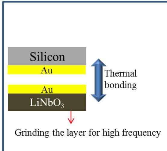
*Figure 2.5.3 First development of bulk LiNbO<sub>3</sub> (30 MHz) and silicon bonding.*
