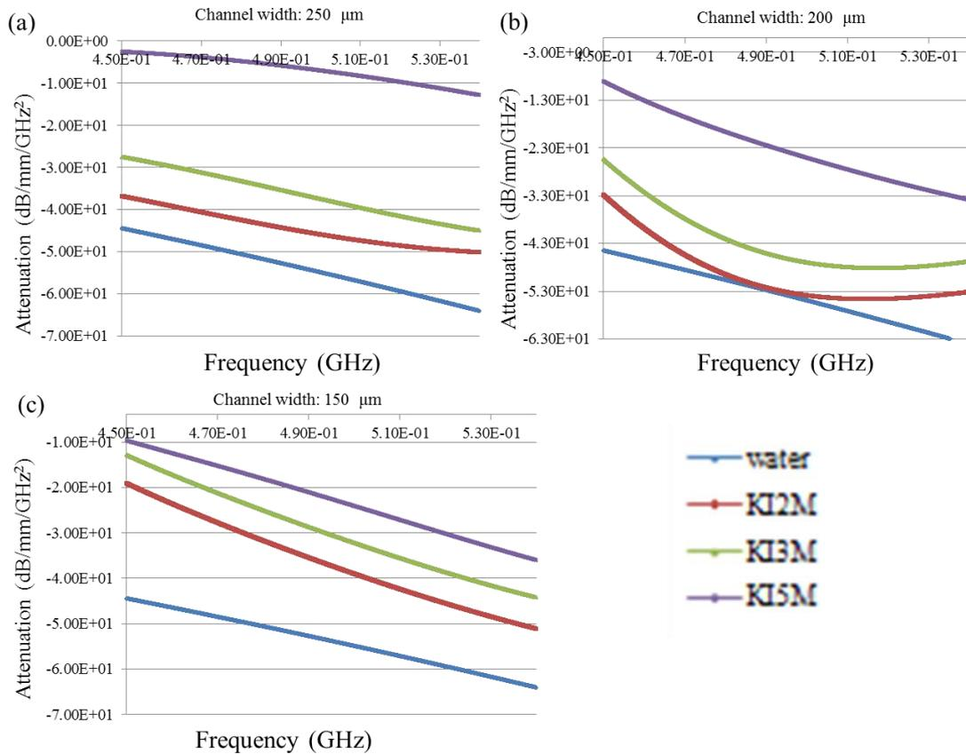
Figure 3.3.5 frequency response of  $S_{12}$  curves for KI solution at 5 mol/L, 3mol/L and 2 mol/L. (a) channel width 250  $\mu\text{m}$ , (b) channel width 200  $\mu\text{m}$ , (c) channel width 150  $\mu\text{m}$ . The frequency ranges from 450 MHz to 540 MHz.
