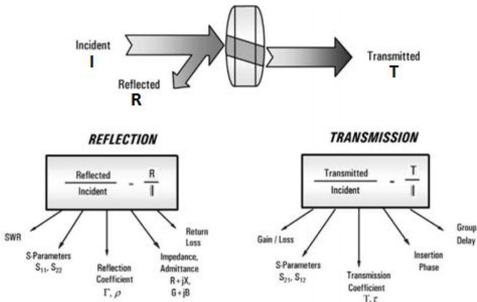
Figure 3.1.1 Principle of measurement of a network analyser [2].
