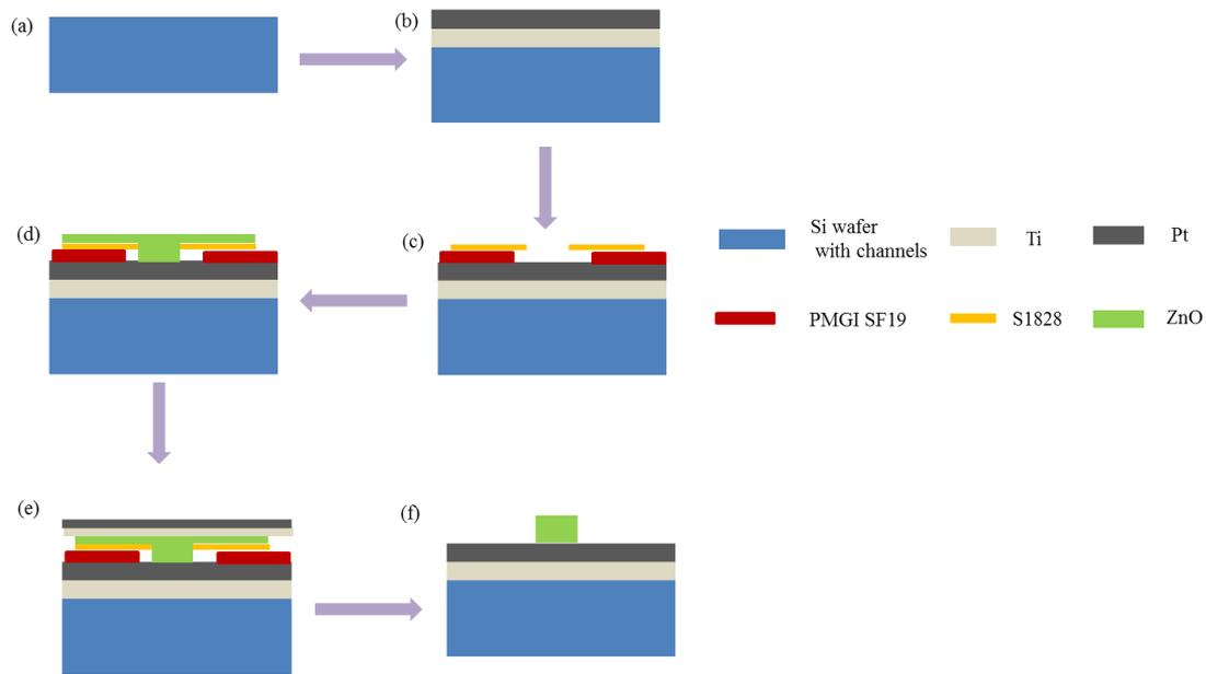
Figure 2.5.4 Procedures for the thin ZnO film fabrication.
