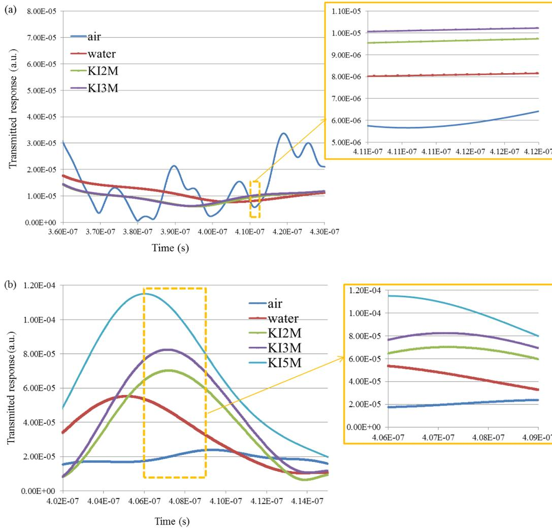
Figure 3.3.3 Transmitted time domain response  $S_{12}(t)$  for sample with two vertical mirrors (a) and sample with one vertical mirror (b) the channel width is  $250\ \mu\text{m}$ . Useful amplitude comparisons are in yellow dash box. Signal characterization in empty channel, deionized water, 2mol/L, 3mol/L and 5mol/L KI solutions respectively.
