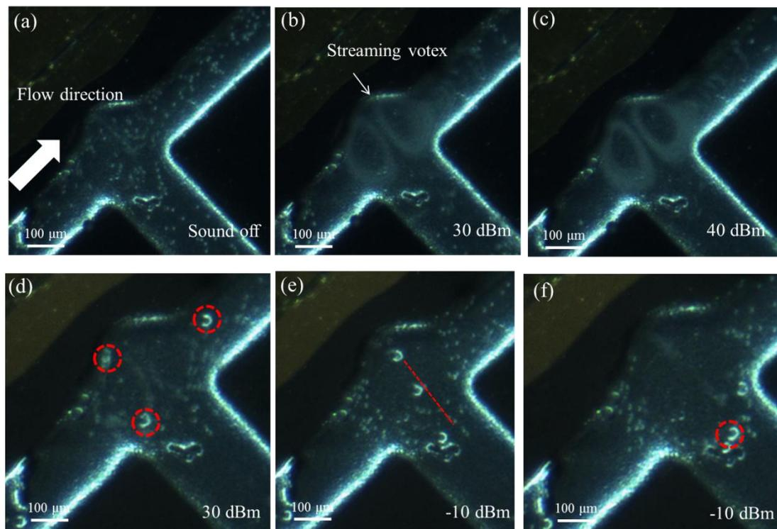
*Figure 3.6.3 Acoustic focusing in lens (Radius 150  $\mu\text{m}$  and focus length 364  $\mu\text{m}$ ) for strong mixing of 9  $\mu\text{m}$  particles (a-c) and separation of 30  $\mu\text{m}$  particles into another branch (d-f) in dynamic flow. Red dash lines indicate 30  $\mu\text{m}$  particles movement. The central frequency of transducer is 600 MHz.*
