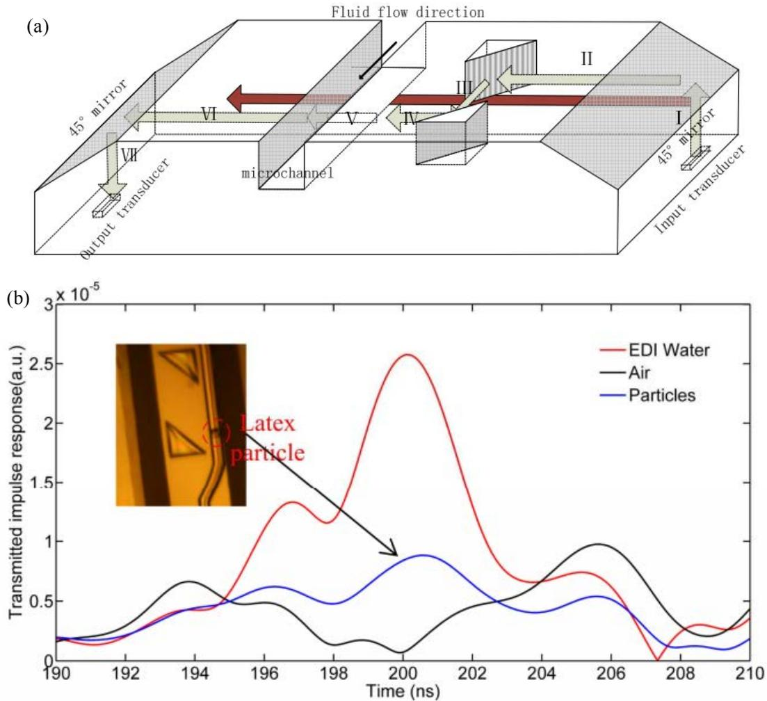
Figure 1.5.3 (a) Schematic illustration of the transmission path in the acoustic guide platform. (b) Modulus of the impulse response ( $S_{21}$ ) for water and particle characterization. (red: channel filled with EDI water; blue: 0.1% concentration of latex particles in EDI water; black: empty channel) [74].
