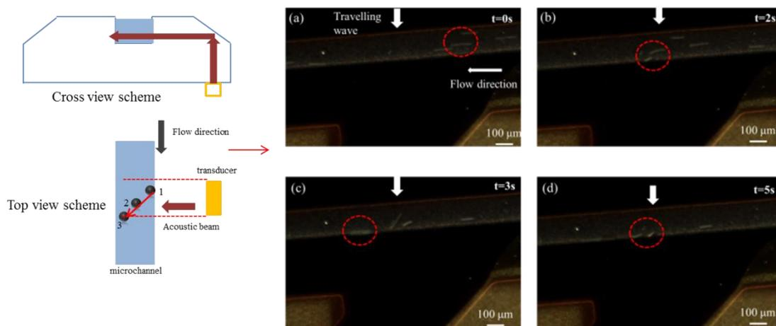
*Figure 3.6.1 particle switch using one travelling wave. (a)  $t=0s$ , particle move along the flow in the middle of the channel, (b)  $t=2s$ , particle started to move perpendicularly to the channel in acoustic field, (c)  $t=3s$ , particle was driven to the down side of the channel by acoustic force, (d)  $t=5s$ , particle move along the flow in the down side of the channel. Input power is 5 dBm, flow rate is  $0.5 \mu L/min$ . Particle was inside the dash circle.*
