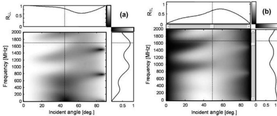
Figure 2.3.2 Reflection coefficient of a longitudinal wave in (a) longitudinal mode  $R_{LL}$  and (b) transverse mode  $R_{TL}$  at silicon – $\text{SiO}_2$  interface (4  $\mu\text{m}$  thickness of  $\text{SiO}_2$  layer) -vacuum interface. (longitudinal wave velocity in  $\text{SiO}_2$ :  $v_L = 6050$  m/s and shear wave velocity  $v_s = 4100$  m/s) [10].
