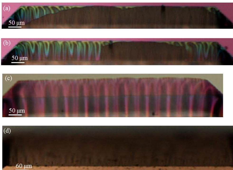
*Figure 2.2.6 Optical mirror observation after wet etch: (a) 10% TMAH+ 10% IPA for 4h etch, (b) 10% TMAH+ 20% IPA for 5h etch, dashed box is the breakaway  $\text{SiO}_2$  mask, (c) 10% TMAH+ 30% IPA for 7h etch, (d) 10% TMAH+ 40% IPA for 9h etch and  $\text{SiO}_2$  removed.*
