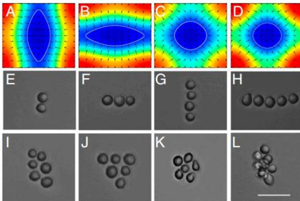
*Figure 1.4.5 Cells assembly in different geometries after acoustic capture. (A–D) Simulation results of acoustic potential distribution in an acoustic well with various amplitudes. The white line indicates an acoustic potential with the same magnitude. (E–H) HeLa cells assembly in a linear shaped acoustic well. (I–K) Single-layer and (L) cell assembled in a spherical shape [57]. Scale bar: 50µm.*
