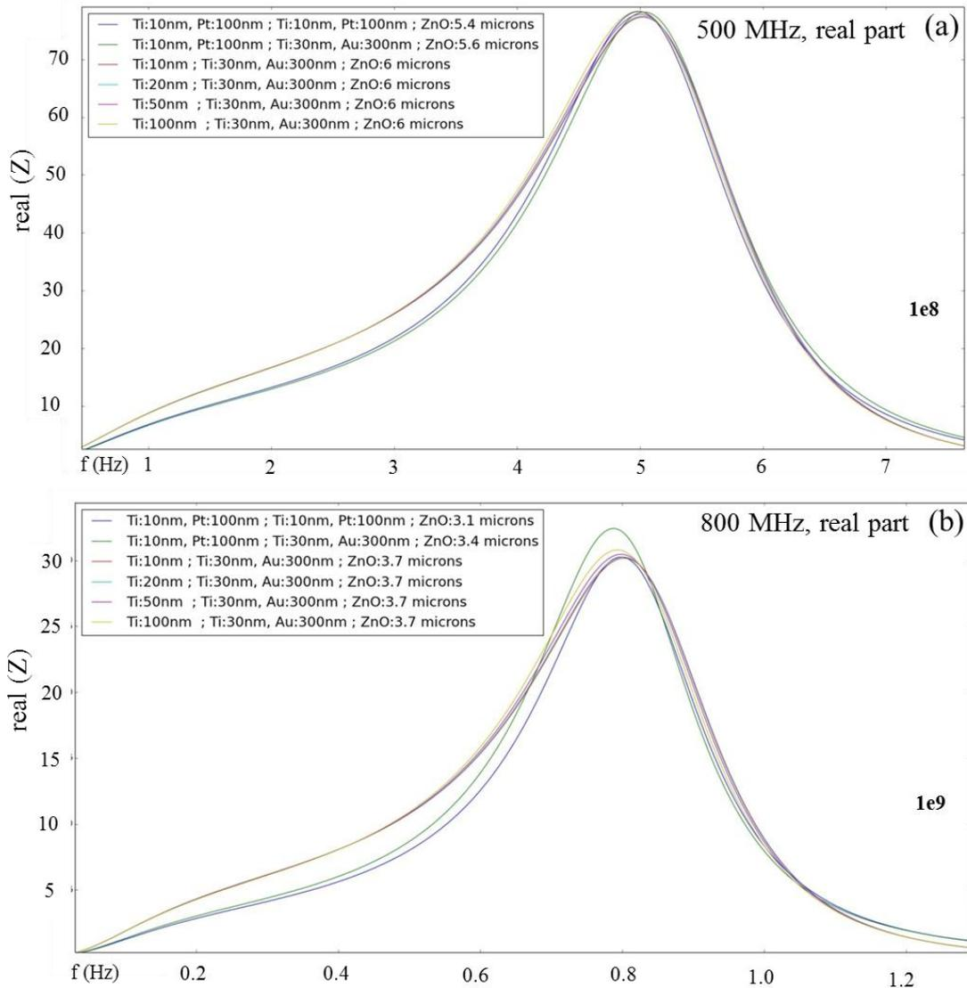
Figure 2.5.11 Impedance influence of ZnO transducer on different ground electrodes and top electrodes. (a) real part impedance at 500 MHz and (b) real part impedance at 800 MHz. In the description of electrodes, the first item is ground electrodes and the second item is top electrodes.
