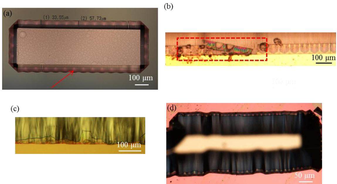
Figure 2.2.8 (a) two hours etching and mirror edge distortion can be observed, (b) 6 hours etching and SiO<sub>2</sub> layer start to split away (dash box), (c) 11 hours etching with visible roughness, d) 4 hours etching and serious deformation.
