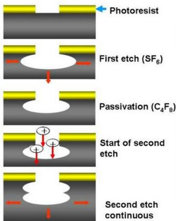
Figure 2.4.3 Step of Bosch methods for Si dry etching [14].
