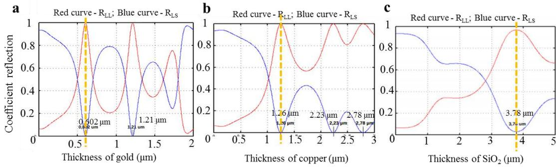
Figure 2.3.4 Simulation for the thickness of the matching at 1GHz harmonic frequency. (a) for gold, (b) for copper and (c) for SiO<sub>2</sub>.
