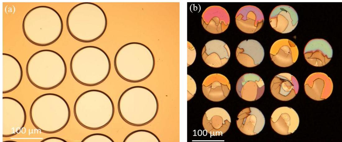
Figure 2.5.5 comparison of a) well deposited 1  $\mu\text{m}$  ZnO film and b) heterogeneous adhesion for 5  $\mu\text{m}$  ZnO film patterns deposition.
