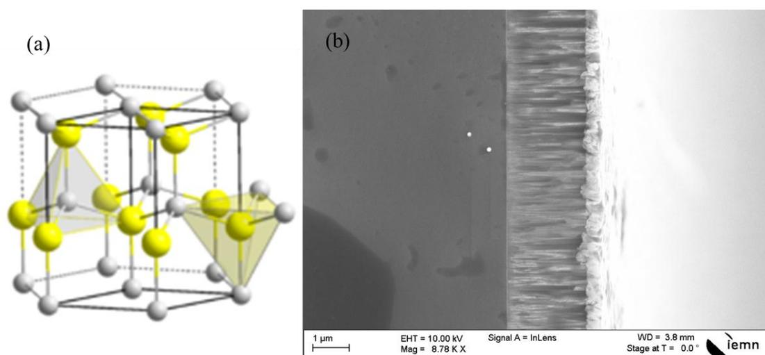
Figure 2.5.1. (a) The wurzite model for ZnO crystalline structure, (b) cross section of SEM for sputtered 2.6  $\mu\text{m}$  ZnO film on Pt ground electrode and gold top electrode.
