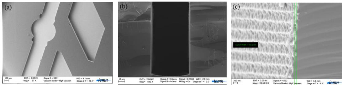
Figure 2.4.4 SEM photos for the survey after DRIE. (a) top view of the channel and vertical mirrors, (b) cross section view of the 140  $\mu\text{m}$  depth, (c) enlarged area of the side wall.
