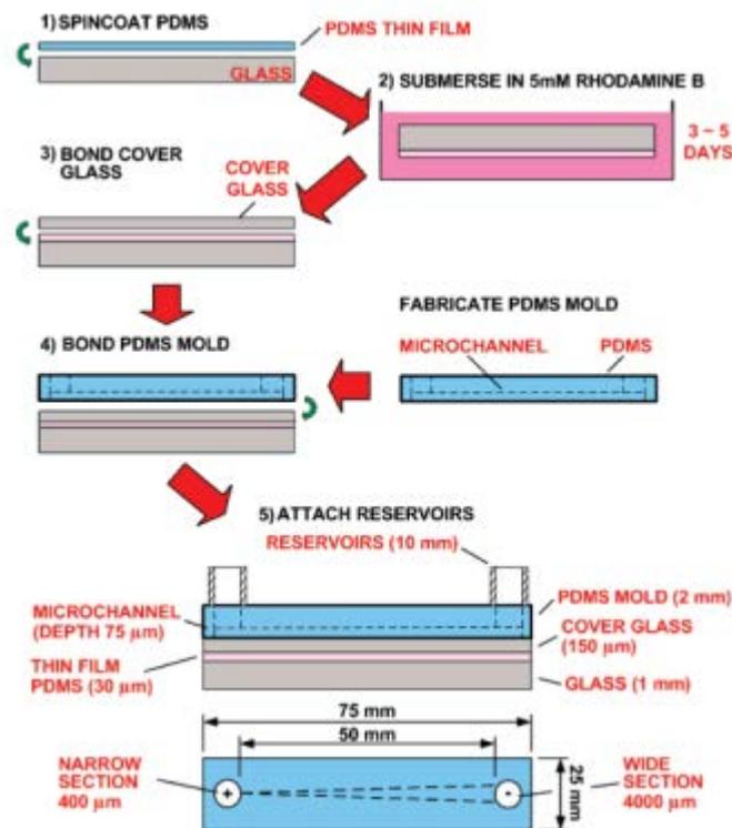
Figure 3.5.2 Schematic of the fabrication process for the Rhodamine B embedded into thin film PDMS and the microchannel.
