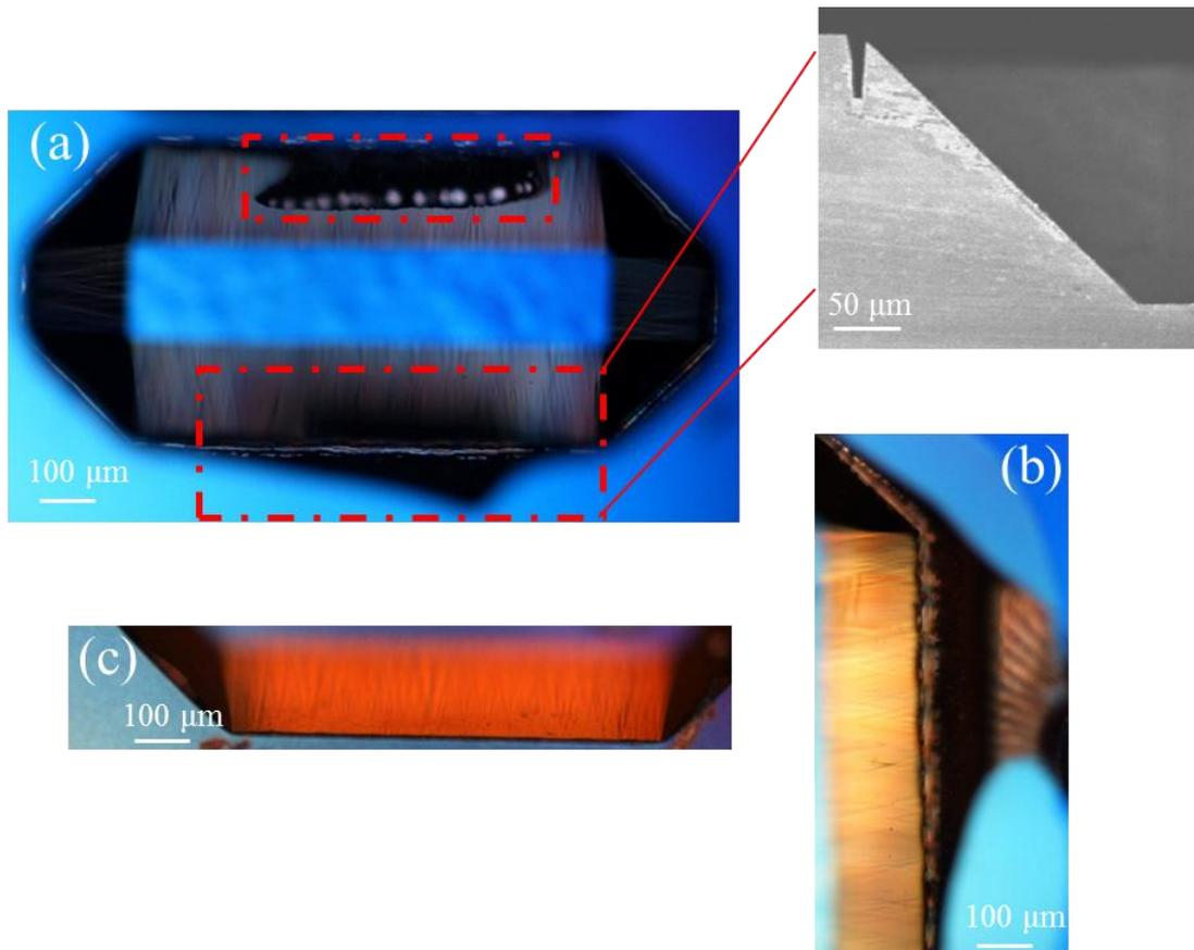
*Figure 2.4.5 Damage and defect by ICP process after treatment (a) on 45° mirror surfaces, enlarged area and SEM of cross-section in dash box, (b) on the edge of the 45° mirror with gold coating, (c) better mirror surfaces with gold coating after improvement of ICP process.*
