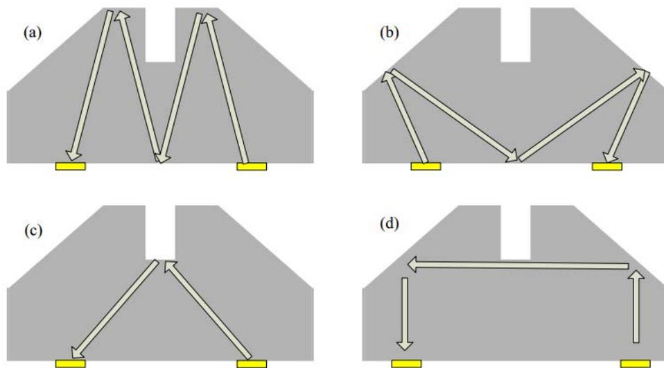
*Figure 3.3.1 Different paths of parasitic acoustic wave propagation. (a) three time reflections by top surface and bottom of the wafer; (b) three time reflections by 45° mirrors and bottom of the wafer; (c) reflection by bottom of the channel; (d) no propagation in the channel.*
