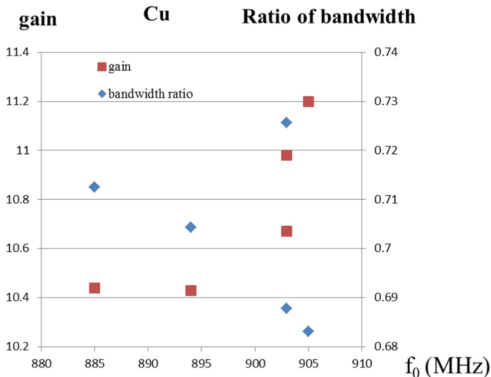
Figure 3.2.6 Gain and bandwidth ratio comparison with 1.26  $\mu\text{m}$  copper layer on mirrors.  $f_0$  is the experimental central frequency of transducer. The frequency ranges from 880MHz to 910MHz.
