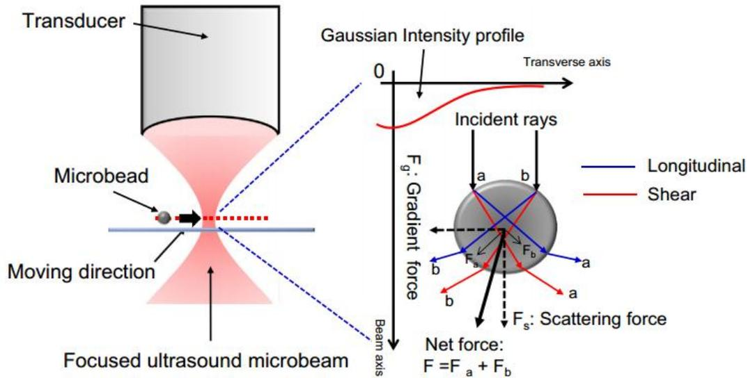
Figure 1.5.1 Illustration of the acoustic mechanism for two incident rays in a Gaussian intensity field trapping a microbead in water [69].
