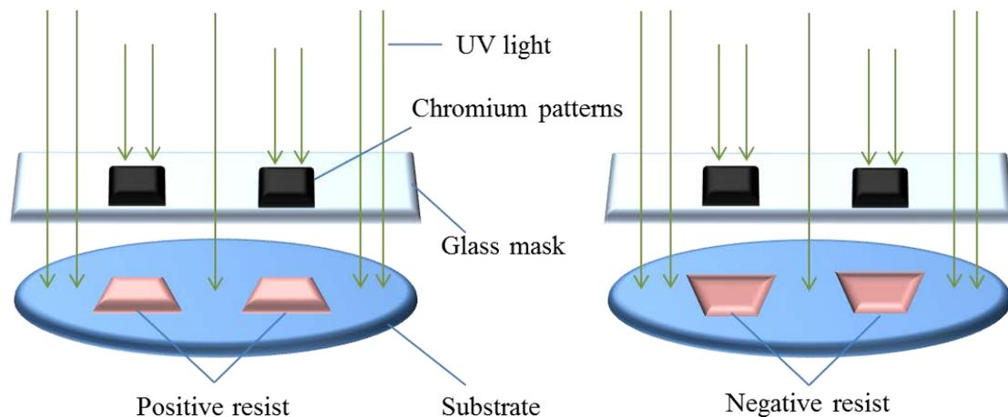
Figure A1 Different edge contour for positive and negative resist after development.
