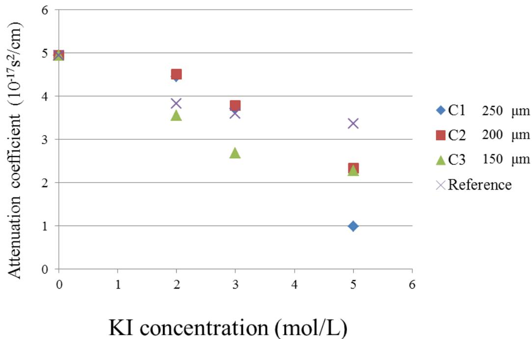
Figure 3.3.4 Calculated attenuation coefficient by time domain echo response for KI solution at 2 mol/L, 3 mol/L, 5 mol/L at 25 °C. C1, C2, C3 are channels with different widths of 250  $\mu\text{m}$ , 200  $\mu\text{m}$  and 150  $\mu\text{m}$  respectively. Reference value for the coefficient was deduced from J. Attal's work [7].
