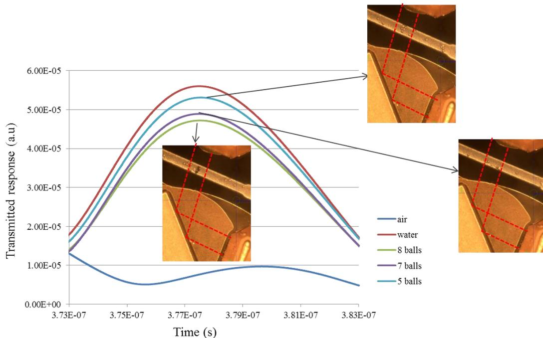
*Figure 3.3.7 Acoustic characterization of particles in 1 vertical mirror system. Different numbers of particles stay in the detection region (red dash lines indicate the acoustic beam propagation) and presented increasing values of attenuation with the number of balls.*
