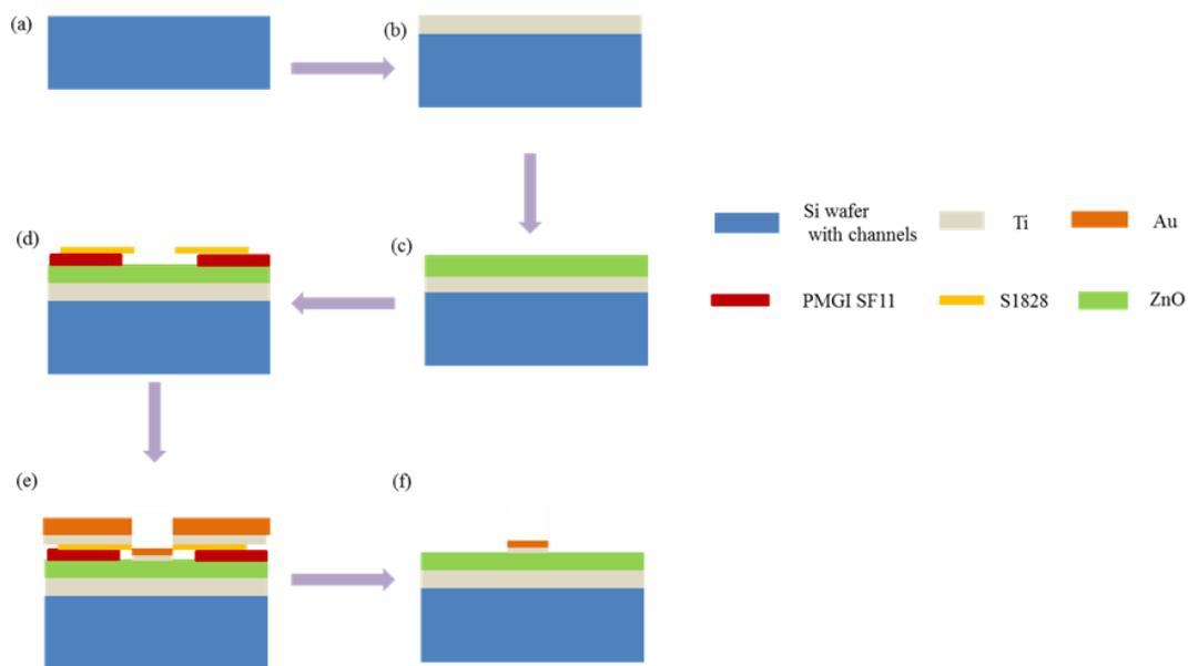
Figure 2.5.6 Improved procedures for the thick ZnO film fabrication.
