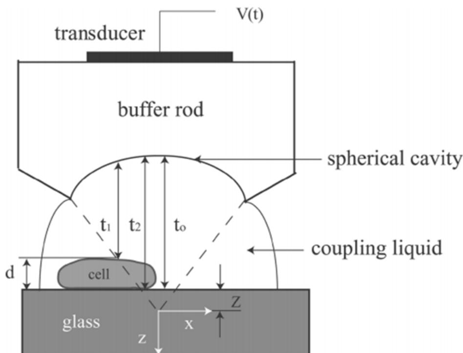
Figure 1.2.1 Setup for a quantitative, time-resolved, acoustic microscopy.
