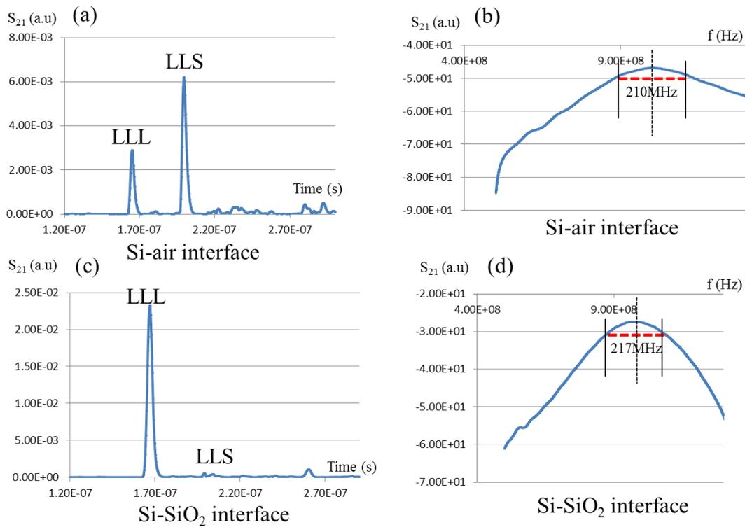
Figure 3.2.4 (a)  $S_{21}$  impulse response in the case of reflection at Si-air interface, (b)  $S_{21}$  frequency response for reflection at Si-air interface, (c)  $S_{21}$  impulse response for reflection at Si- SiO<sub>2</sub> interface, (d)  $S_{21}$  frequency response for reflection at Si- SiO<sub>2</sub> interface. The width of dash line shows the -3dB bandwidth value.
