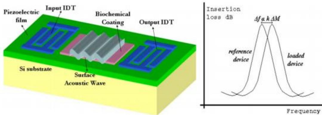
Figure 1.2.2 Sketch of a typical SAW-based bio/chemical sensor using the frequency-shift based response. The center frequency shift from the reference to the loaded devices when there is a change in the mass that modifying the SAW propagation [29].
