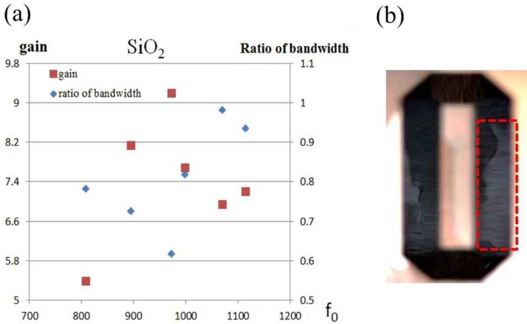
Figure 3.2.5 (a) Gain and bandwidth ratio comparison with a constant  $3.8\mu\text{m}$   $\text{SiO}_2$  layer on the mirrors, (b)  $\text{SiO}_2$  film partially damaged in dash box.  $f_0$  is the experimental central frequency of the transducer. The frequency extends from 800MHz to 1200MHz.
