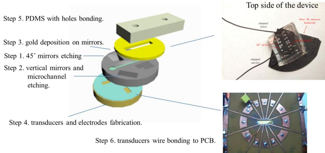
*Figure 2.1.3 Identified process of lower frequency device.*
