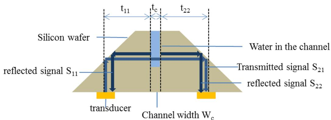
Figure 3.5.5 time interval in the acoustic propagation.  $t_{11}$ : time for acoustic wave from the generator to the microchannel,  $t_c$ : time for acoustic transmission in the water with the channel,  $t_{22}$ : time for acoustic wave from the channel wall to the receiver.  $W_c$  is the channel width.
