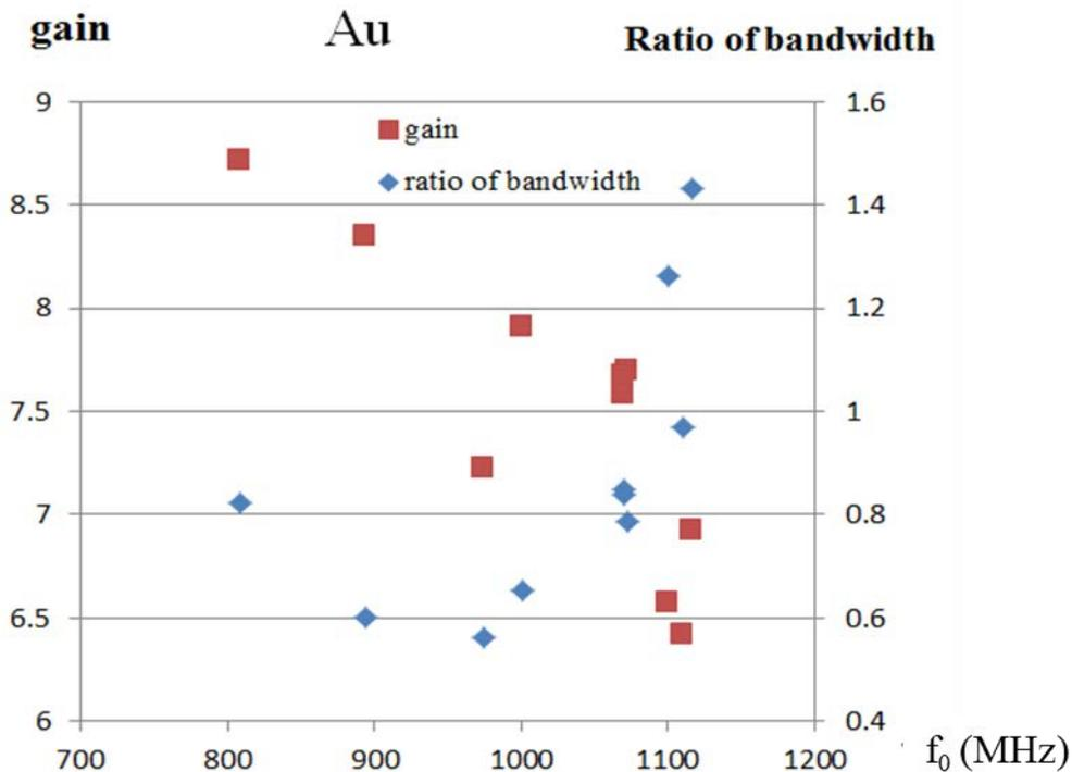
Figure 3.2.7 Data graph of gain and bandwidth ratio comparison with 800 nm gold layer on mirrors.  $f_0$  is the experimental central frequency of transducer. The frequency ranges from 800MHz to 1200MHz.
