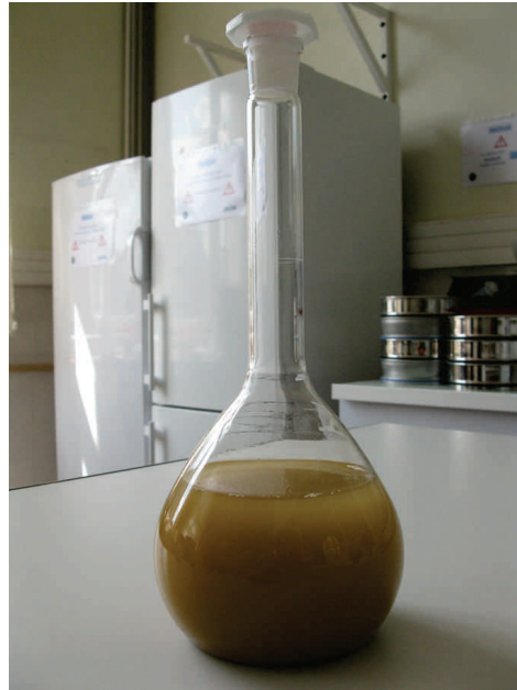
Figure 2.33 – Clay suspension used to modify the NVSS fraction of the sludge samples.
