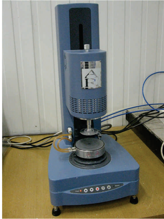
Figure 2.10 – Rheometer used for the rheological measurements.
