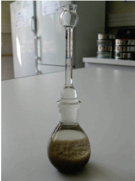
Figure 2.32 – Pycnometer containing an activated sludge sample.
