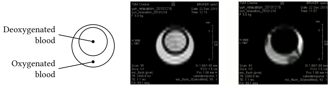
Figure 4.1: Contrast optimization: both pictures were taken using the same setup of two tubes, the inner one containing deoxygenated blood and the outer one containing oxygenated blood. The left-hand picture is the picture obtained with no contrast optimization; the right-hand picture is contrast-optimized by saturating the inner sample.
