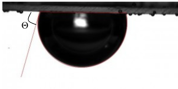
Figure II.2: Example of contact angle measurement by the captive bubble technique
