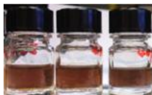
Figure I. 2 Photographs of resulting Ag NP solutions synthesized at 40 °C for 10, 15 and 20 minutes (from left to right), respectively.
