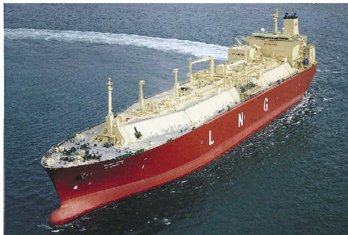
Figure 1.1: LNG tanker with Membrane containment systems.
