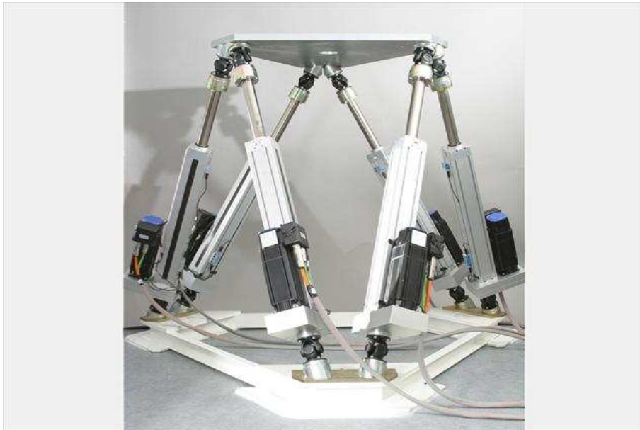
Figure 3.37: The MISTRAL hexapod from http://www.symetrie.fr .
