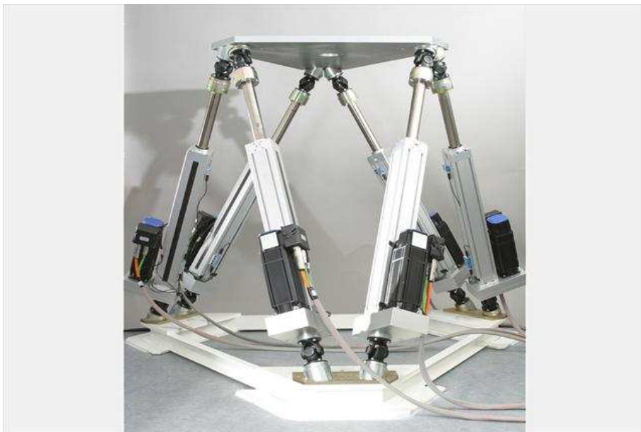
Figure 3.37: The MISTRAL hexapod from http://www.symetrie.fr .
