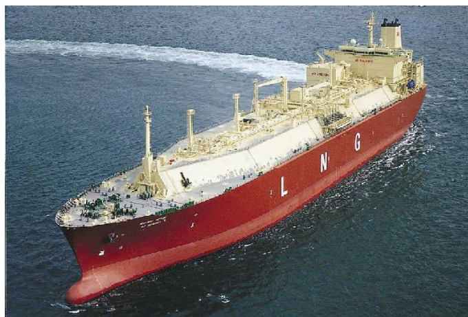
Figure 1.1: LNG tanker with Membrane containment systems.
