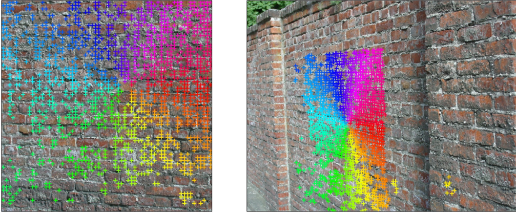
Figure 3.8 – Matching result between two images with repetitive textures. Nearly all output correspondences are correct. Wrong matches are due to occluded areas (bottom-right of the first image) or situations where the deformation tolerance of DeepMatching is exceeded (bottom-left of the first image).
