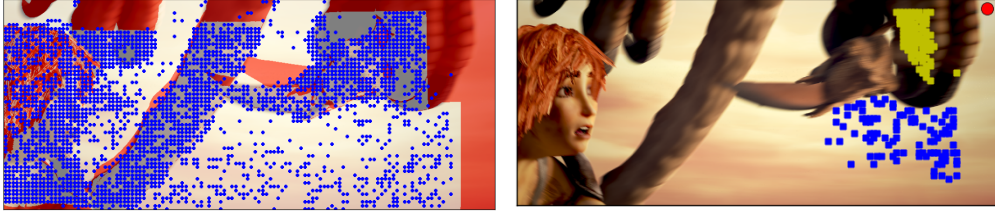
Figure 4.6 – Left : Match positions returned by DeepMatching [Weinzaepfel et al., 2013] are shown in blue. Red denotes occluded areas. Right : Yellow (resp. blue) squares correspond to the 100 nearest matches with a Euclidean (resp. edge-aware geodesic) distance for the occluded pixel shown in red. All neighbor matches with a Euclidean distance holds to a different object while the geodesic distance allows to capture matches from the same region, even in the case of large occluded areas.
