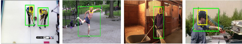
Figure 8.3 – Examples of bounding boxes (green) estimated from annotated joints and head (yellow) on the MPII Human Pose dataset.
