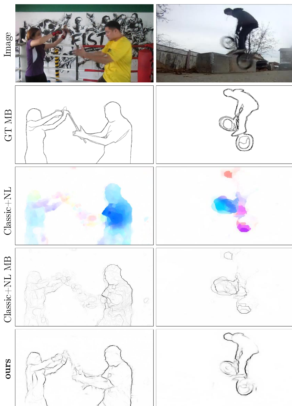
Figure 5.9 – Example results from the YMB dataset with, from top to bottom: images, annotated motion boundaries, flow estimation using Classic+NL [Sun et al., 2014b], norm of the flow gradient (Classic+NL MB), and the motion boundaries estimated by our method (ours).
