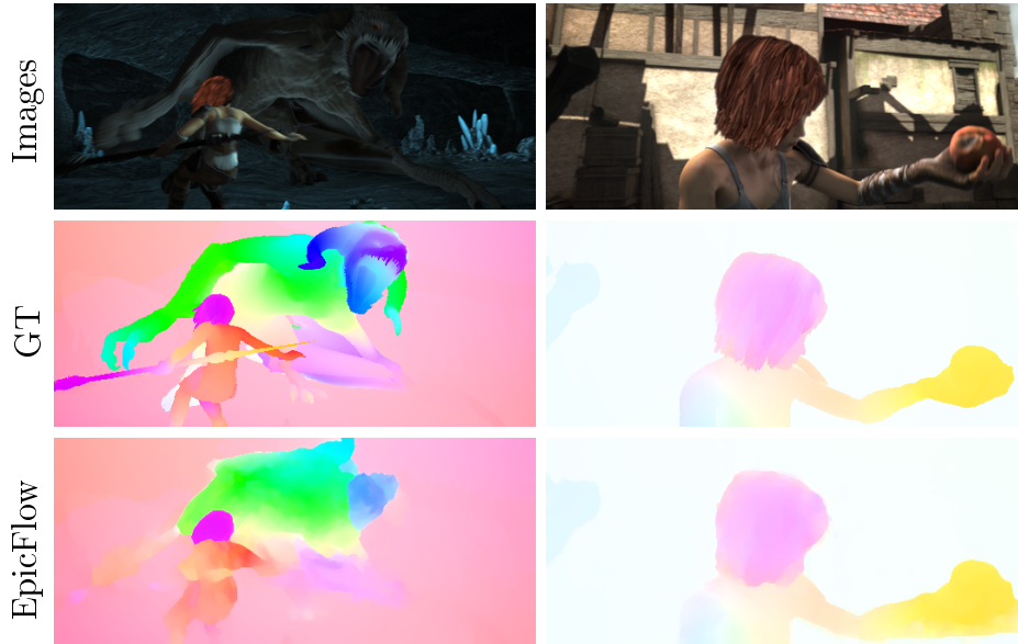
Figure 4.9 – Failure cases of EpicFlow due to missing matches on spear and horns of the dragon (left column) and missing contours on the arm (right column).
