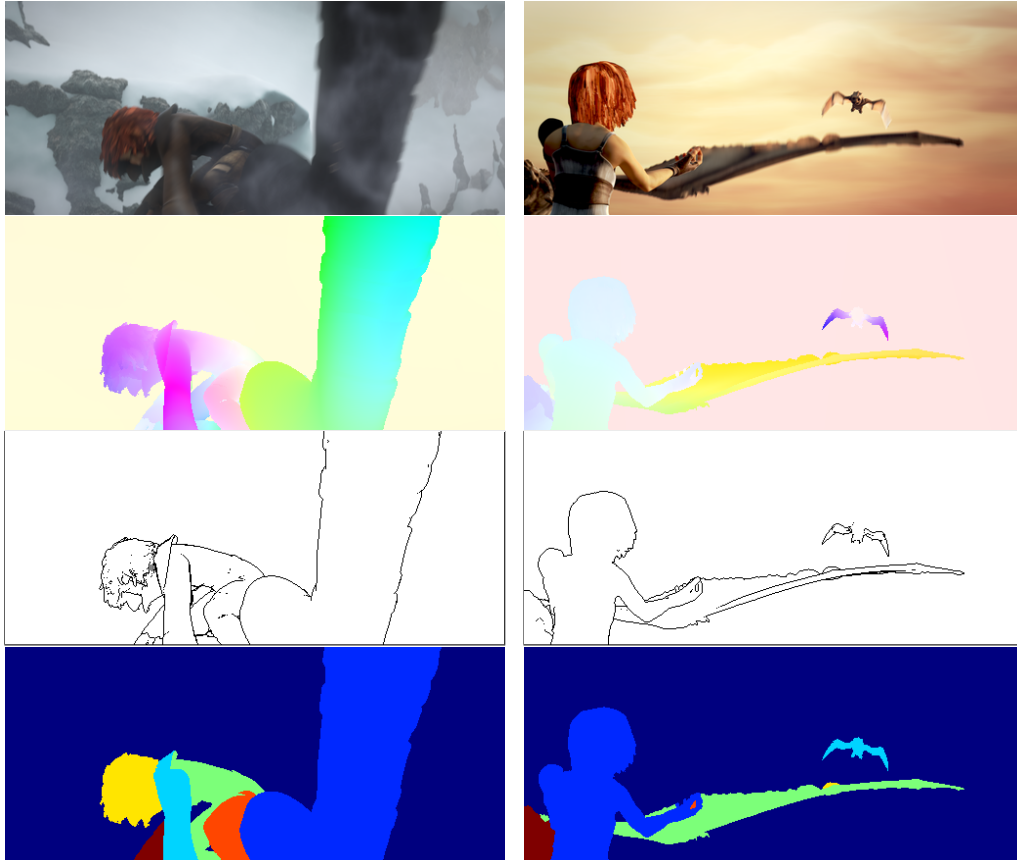
Figure 5.5 – From top to bottom: example images, corresponding ground-truth flow, ground-truth motion boundaries and motion layers used for training.
