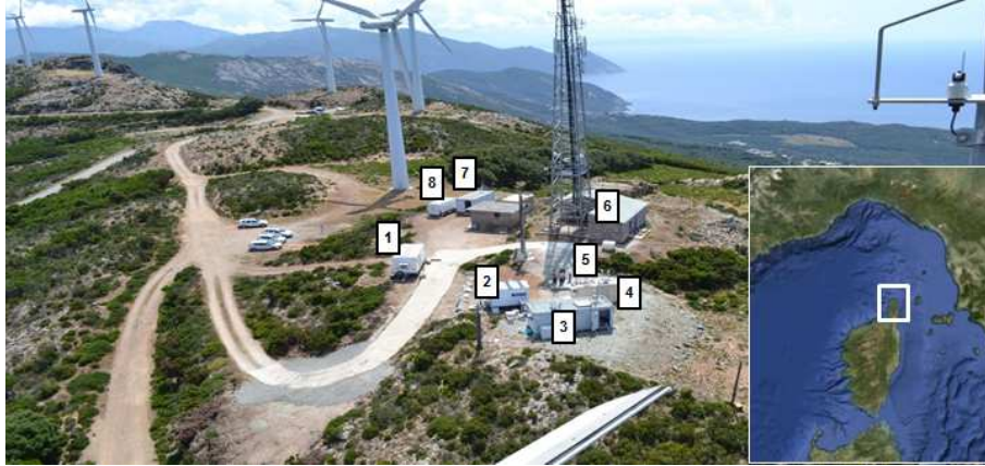
Figure 5.1: Field site of Ersa windfarm ( 42.97^\circ N, 9.38^\circ E, altitude 533 m) located in Corsica, France, where the ChArMEx-CARBOSOR campaign took place. Measures location: 1. Trace gases with PTR-MS, online and offline chromatography; 2. OH reactivity; 3. \text{NO}_x , \text{O}_3 , aerosols composition and black carbon; 4. Meteo and particles microphysics; 5. HCHO, trace gases and radicals; 6. CO, \text{CO}_2 , \text{CH}_4 ; 7. Trace gases and particle filters; 8. Particles physics. The photo was taken before the start of the campaign (cars parked nearby).
