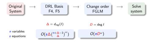
Figure 1.1: Strategy of resolution for a system of dimension 0
