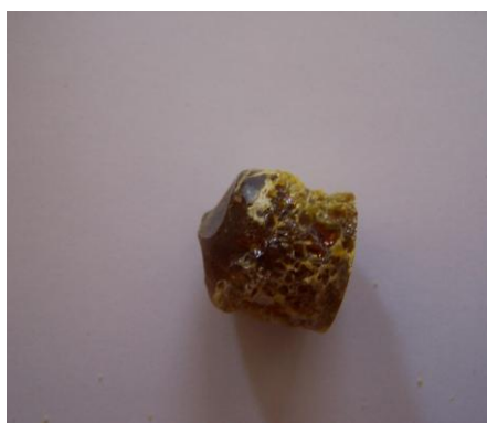
Figure 79: GeS 3 sample crystallised during fiber drawing attempt.
