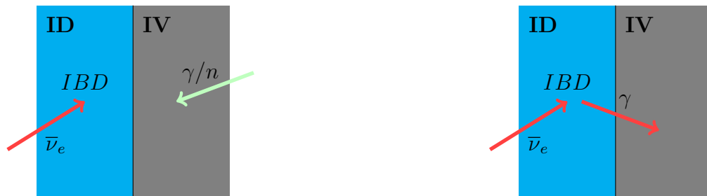
FIGURE 5.13: Illustration of IBD in coincidence with IV events. On left is the schematization of accidental coincidence, and on right the correlated coincidence.
