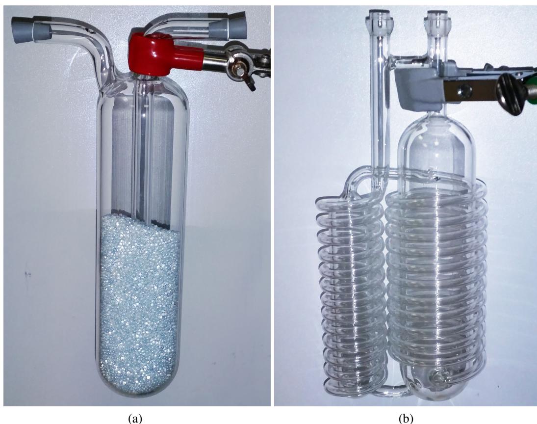
Figure C.6: Pictures of the two type of cryogenic traps deployed in Antarctica and used at LSCE: C.6a single trap filled with glass balls to increase the surface where the vapour can condensed and C.6b double trap without glass balls but with an efficient architecture still totally traps the moisture for flow below 6 L.min^{-1} .
