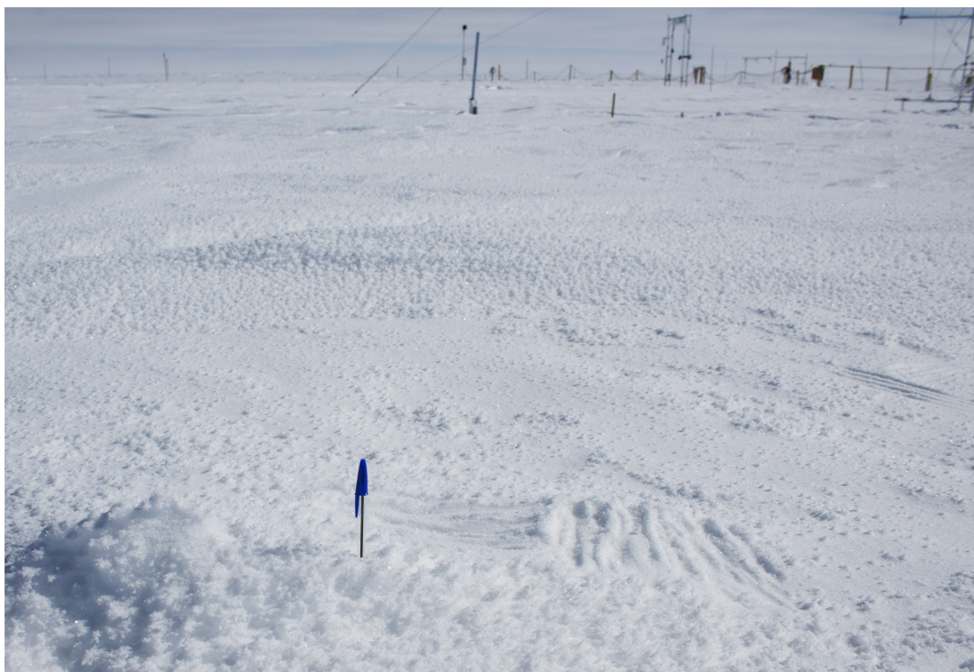
Figure 7.2: Impact of the surface snow sampling, approximately 20 per 10 cm of snow are gathered. The surface conditions vary a lot at the meter scale with the presence or not of frost hoar.
