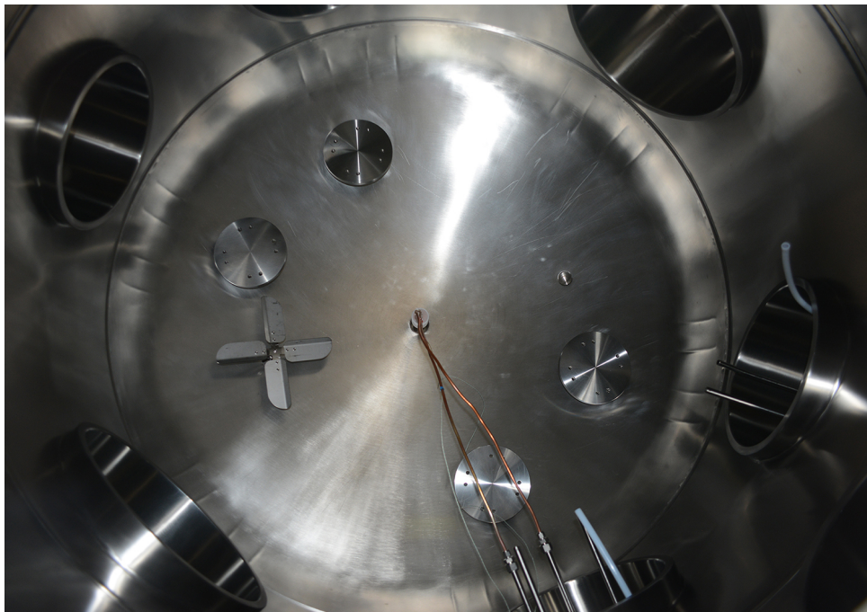
Figure 5.3: Picture inside the cloud chamber CESAM: two copper inlets pump air at different heights of the cold plate here covered with frost. No other sign of condensation is visible on the rest of the cloud chamber.
