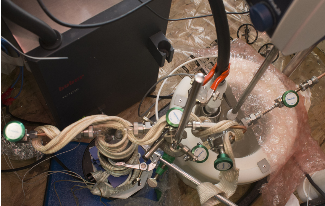
Figure 6.4: Picture of the cryogenic trapping set up in the Snow Shelter at Dome C: while a trap is connected to the outside air, the previous one is heated to detrap the water from the glass balls and transfer it into a small phial
