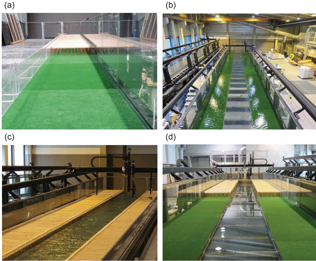
Figure 2.6: Flume viewed from upstream in configurations (a) MW, (b) CM, (c) CW and (d) viewed from downstream in configuration CWM.
