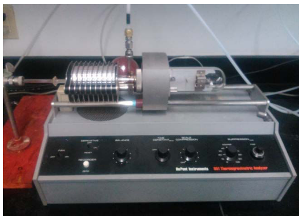
Figure II-13: Dupont Thermogravimetric Analyzer (TGA) used for methane cracking tests over a bed of biochars
