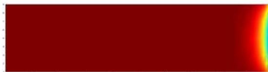
Figure V-11: Hydrogen concentration profile into a micropore: d_{pore} = 1.4 nm, L_{pore} = 14 nm, 1 st iteration (1s)
