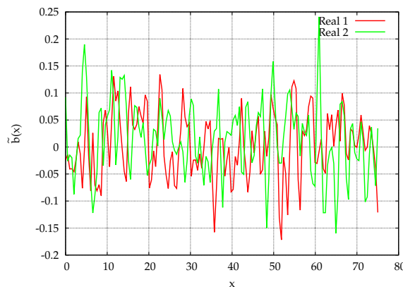
Figure 3.10: SV. Added noise as a function of space with \alpha = 10^{-1} and N_x = 150 for two different realizations.
