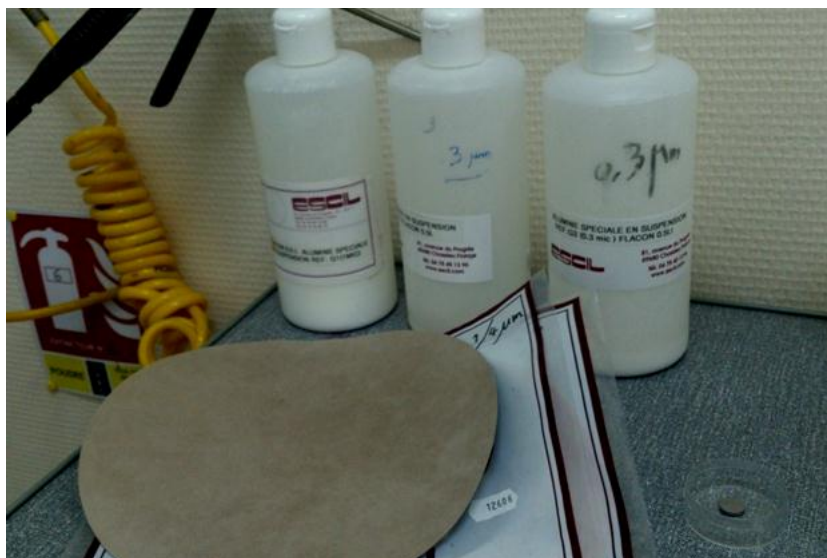
Figure 2-16 Polishing cloth, and suspensions for the Al-Cu alloy samples employed in this thesis.
