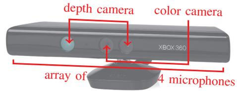
Fig. 1. Kinect sensors
