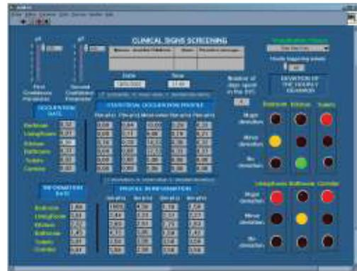
Figure 9. The distribution of Activity rhythms is compared in real time to the model and it raises alarms in case of abnormal deviation.
