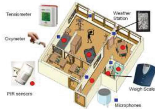
Figure 5. The experimental platforms AILISA used PIR sensors (red dots) distributed in the environment and wirelessly connected to a local CAN network.
