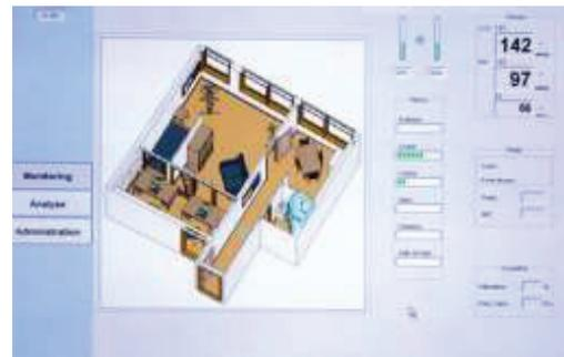
Figure 6. On the monitoring screen are displayed in real time the levels of activities in each room, together with the physiological parameters last recorded.
