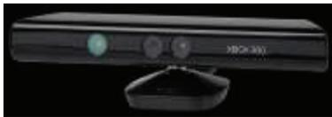
Figure 4. The Kinect (Microsoft Inc., Nov. 2010) is a motion sensor to be used as a remote control for the Xbox 360 video game console.
