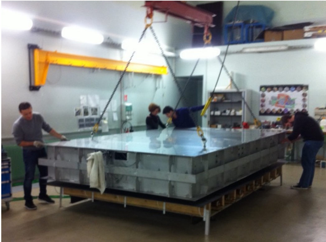
Figure 3.24: The muon veto in the Ariane Hall at the LPSC. Its dimensions are 396 \times 240 \times 25.9 \text{ cm}^3 and it's filled with purified water.
