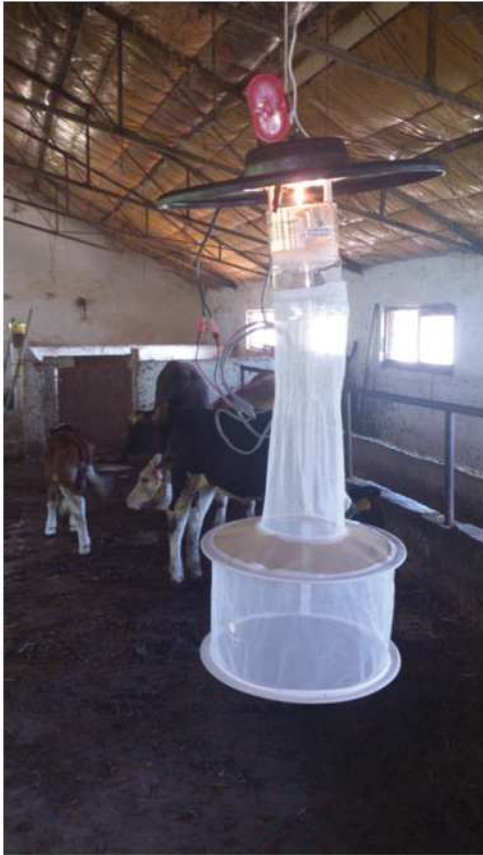
Fig. 1. Light trapping for sand flies in Turkey (Photo credit: Filiz Gunay & Gizem Oguz).
