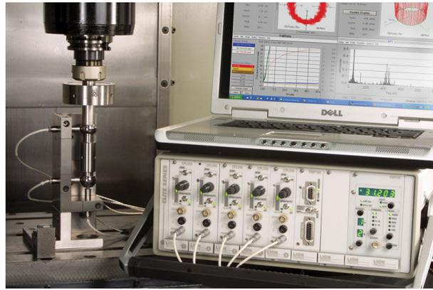
Figure 1.21 – Spindle Error Analyser [IBSPE, 2014].
