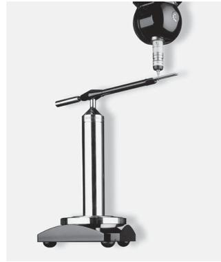
(b) Machine Checking Gauge (MCG) [Renishaw, 2016c].
