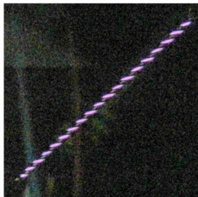
Figure 103: Glowing discharges from a twisted pair of enameled wire connected to the convert output, at low pressure
