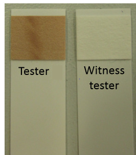
Figure 104: Ozone test in the vacuum chamber, with converter running and twisted pair of enameled wire
