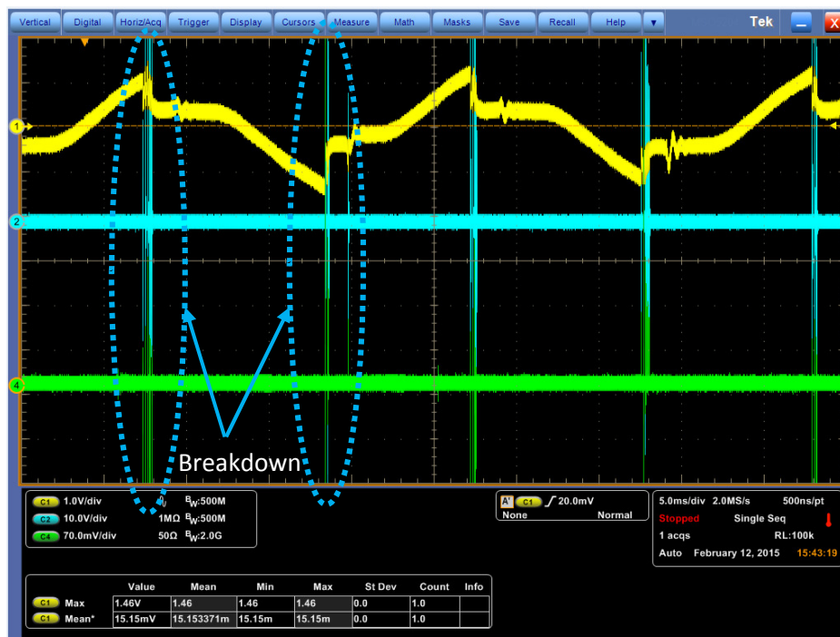
Figure 66: Voltage waveform during a breakdown event on the male part of the connector subject to AC voltage (phase-to-phase test). Channel 1: Power source (kV). Channel 2: Rogowski coil without filter. Channel 4: Coaxial cable without filter
