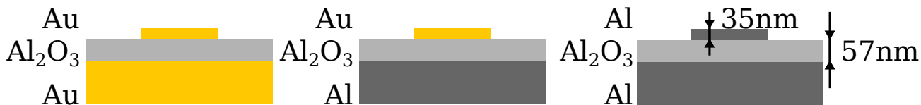
Figure 2.23 – Different materials combinations used for the patch antennas.
