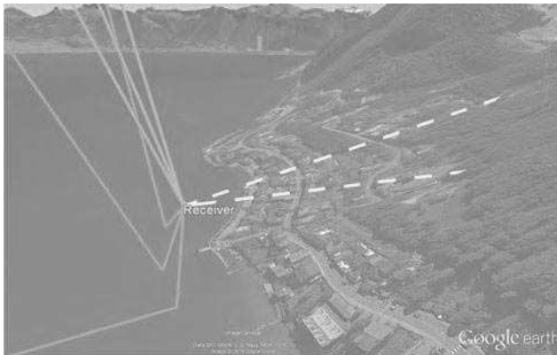
Figure 15. Influence of the topography – direct and reflected waves are displayed (topography amplified by a factor of 3). Yellow lines: direct waves, sphere approximation algorithm; green lines: direct waves, taking a DEM into account; blue lines: reflected waves, sphere approximation algorithm; red lines: reflected waves, taking a DEM into account. It can be noticed that some yellow and blue lines (direct and reflected waves, sphere approximation algorithm) go through the mountain (reflection points having been calculated inside the mountain), whereas any red or green lines (direct and reflected waves, integrating a DEM) go through it.
