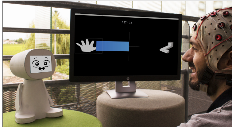
Figure 31 – Illustration of a participant taking part in a Mental-Imagery based Brain-Computer Interface (MI-BCI) training process during which he learns to perform different MI-tasks (here, imagining a left-hand movement) to control the system. Along the training, PEANUT provides the user with social presence and emotional support adapted to his performance and progression. This photo is an illustration ; the real experiments were performed in an experimental room, and PEANUT was providing interventions only between the trials - not during the trials so that it does not disturb the participant while the latter was performing the MI-tasks.
