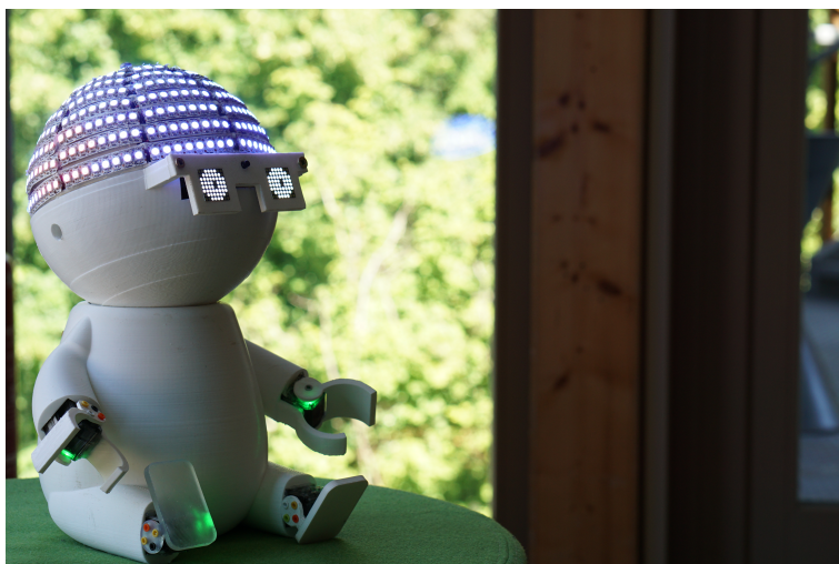
Figure 36 – Photo of TEEGI. TEEGI enables the visualisation of brain patterns associated to specific tasks such as the execution of motor movements.
