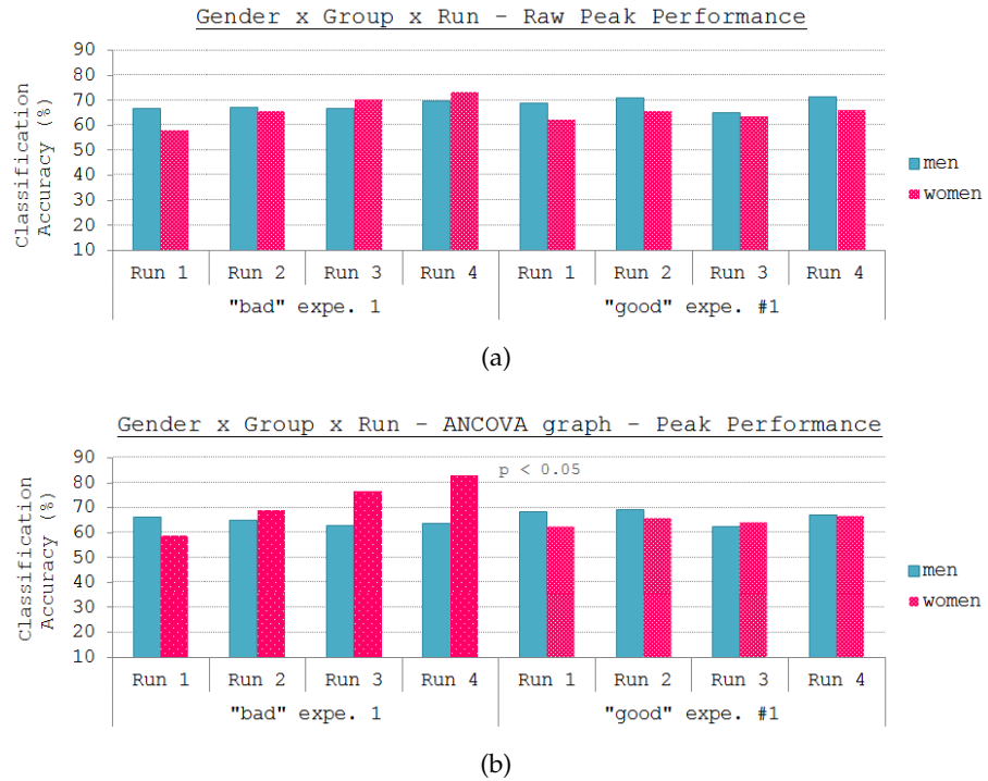
Figure 43 – (a) Graph representing participants’ raw MI-BCI peak performance (i.e., without the ANCOVA correction) as a function of their gender, of their group and of the run; (b) Graph representing the ANCOVA results for the Gender*Group*Run interaction ( p < 0.05 ), considering the Mental Rotation Scores as a covariable. When considering the performance independently from the mental rotation scores, it can be noticed that women from the group "bad" [dark red on the left] improve in terms of performance across the runs while all the other participants do not.
