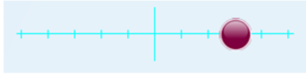
Figure 49 – Visual feedback with current feedback symbolising the recognition of a right hand MI, at level 3/5.
