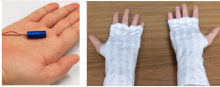
Figure 50 – Left: A vibration motor. Right: Our gloves with 10 embedded motors (5 per hand). In the tactile feedback condition, individual motors are activated to represent the classifier output.
