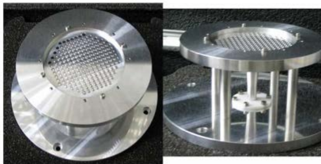
FIGURE 1.25: EBG resonator feed for side-fed offset cassegrain antenna in Ka-band [41].
