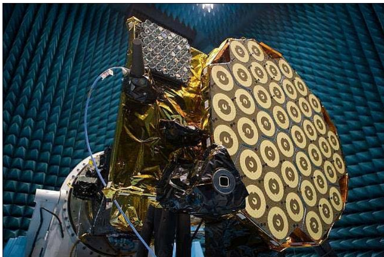
FIGURE 1.9: Earth-Facing Panel of GIOVE-B showing the navigation antenna and the LRR panel.
