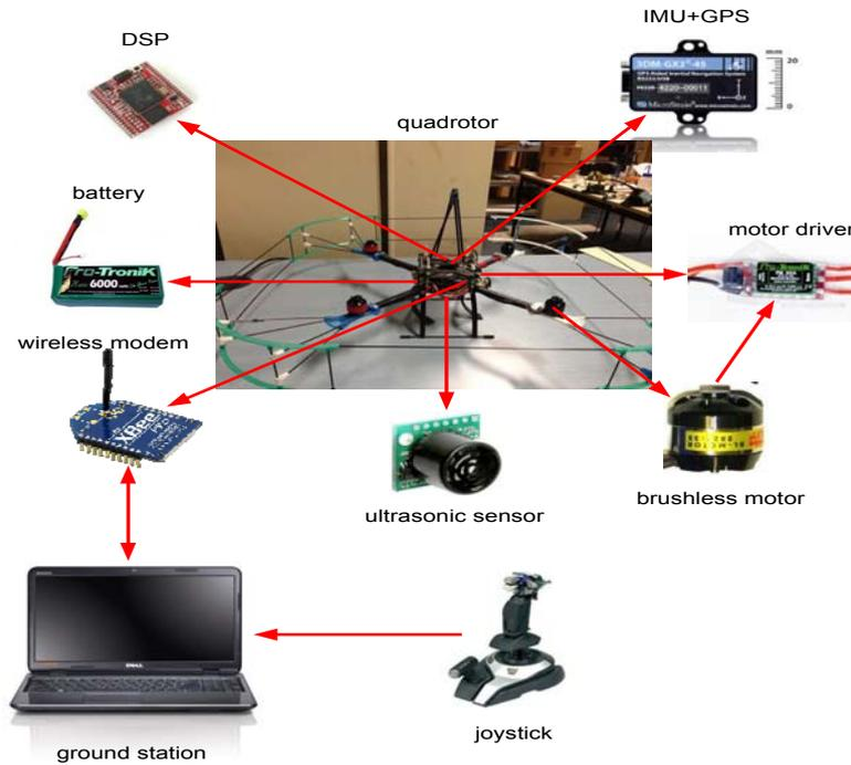
Figure 2-2: Quadrotor main components.
