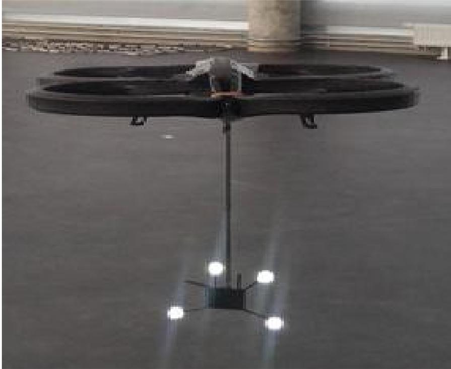
Figure 6-1: Experimental platform for a quadrotor with a cable suspended load.
