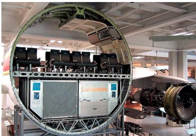
**Figure 7** – Cross-section of an Airbus A300 fuselage. We remark the circular holes in the cantilever. Image released under Creative Commons license 2.5
