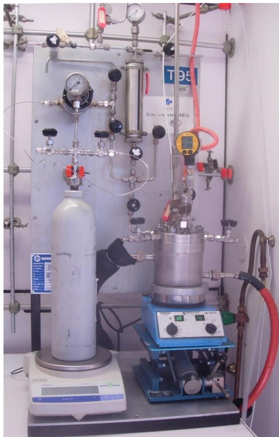
Figure 10. Oligomerisation unit T095 used for this study (on the left, ethylene ballast on a balance, on the right: reactor)
