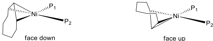
Figure 17. Position of the COD in the complexes that can be located above or below the P_1, Ni, P_2 coordination plane according to the solid state crystal structures of zwitterionic cationic nickel complexes.
