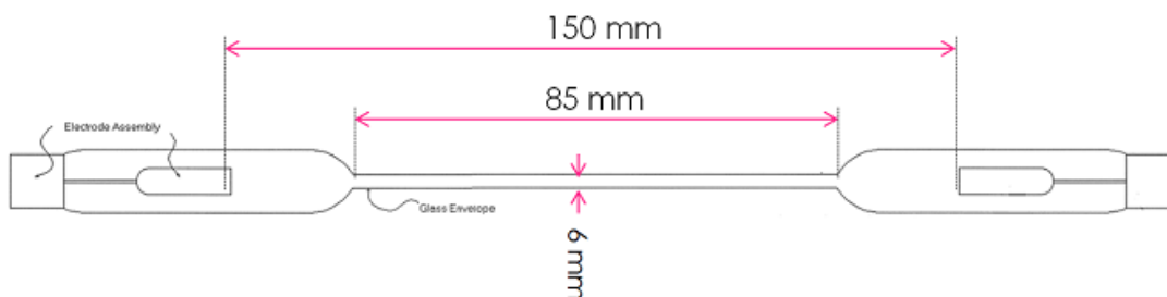
Figure 4.4 The discharge tube used in our experiment. The length between electrodes is 150mm.
