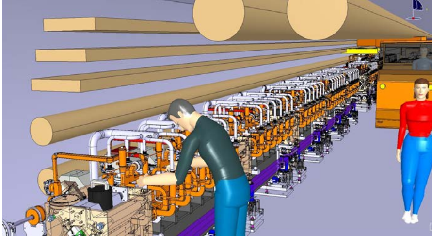
Figure 2-3: 3D simulation of Modules in series in the CLIC tunnel
