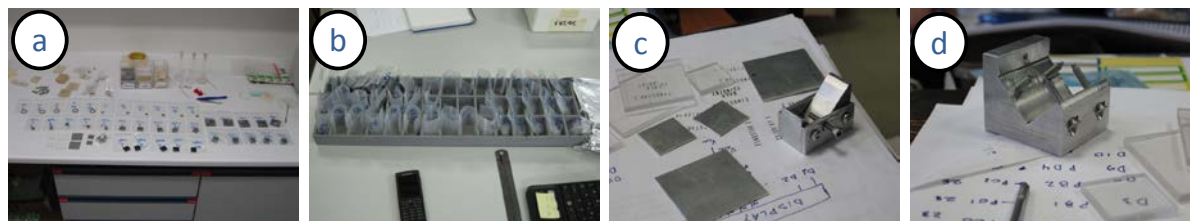
Figure 6-9: a, b) Specimen before the irradiation sessions, c, d) Support configuration for the specimen assembly.
