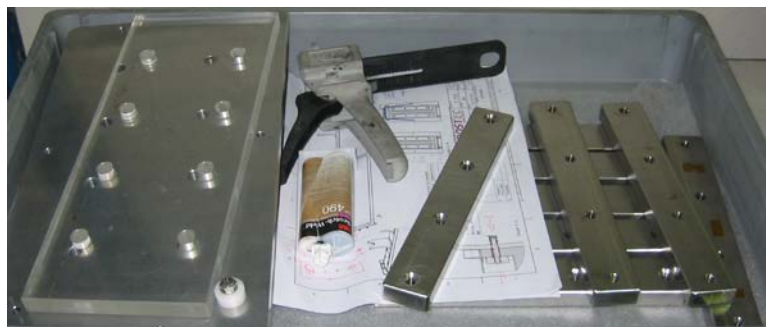
Figure 4-15: Girder metal plates for cradle fixation
