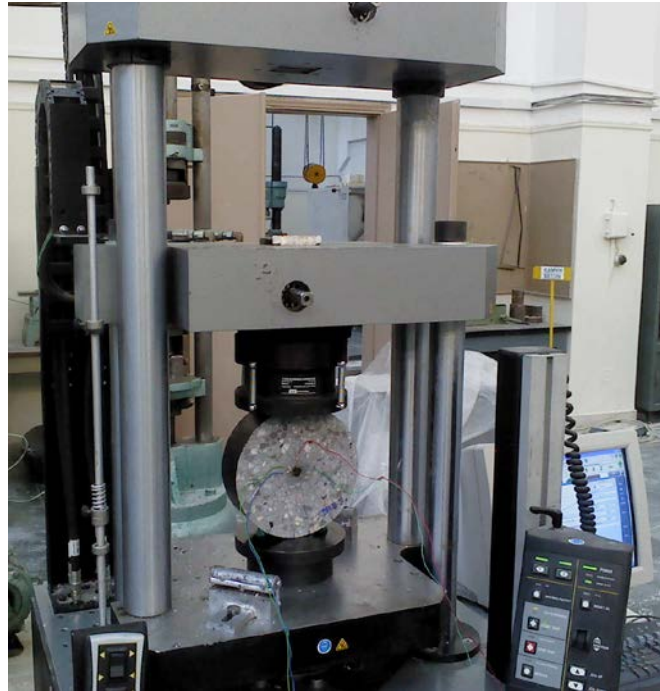
Figure 6-28: Epument sample in the Brazilian disc test setup
