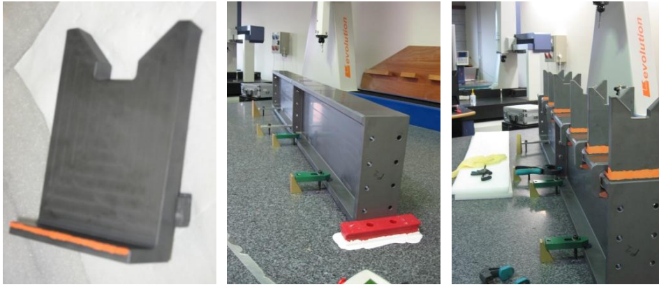
Figure 4-14: Case A monolithic parts made of SiC
