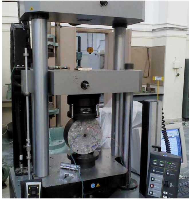
Figure 6-28: Epumet sample in the Brazilian disc test setup
