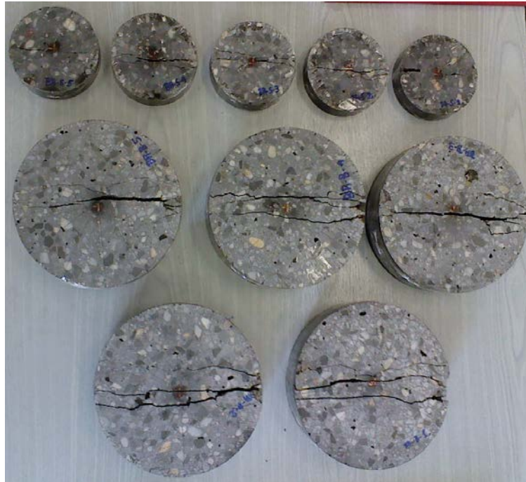
Figure 6-39: Epument samples after the Brazilian disc tests
