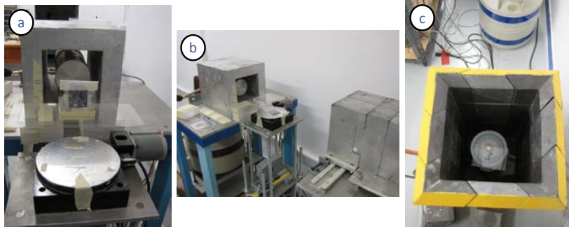
Figure 6-11: High purity Germanium detector measurements (post-irradiation measurements) for the radio-activation and characterization of the specimen
