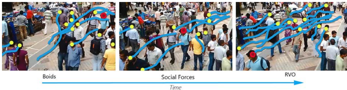
Figure 5.11 – Our mixture motion model can accurately compute the trajectories in real time. We highlight different motion models (Boids, Social-Forces, or reciprocal velocity obstacles) used for the same pedestrian (marked in red) over different frames. We believe that it is not possible to model the trajectory of all pedestrians based on a single, uniform model. Instead, we adaptively choose the best-fit model for every pedestrian in the scene that can be adapted to the environment or the crowd conditions.
