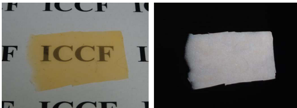
Figure 118 Photographs of free-standing 2 wt. % mixed QDs-silicone composite films (left) under normal light and (right) under a 365 nm UV illumination.
