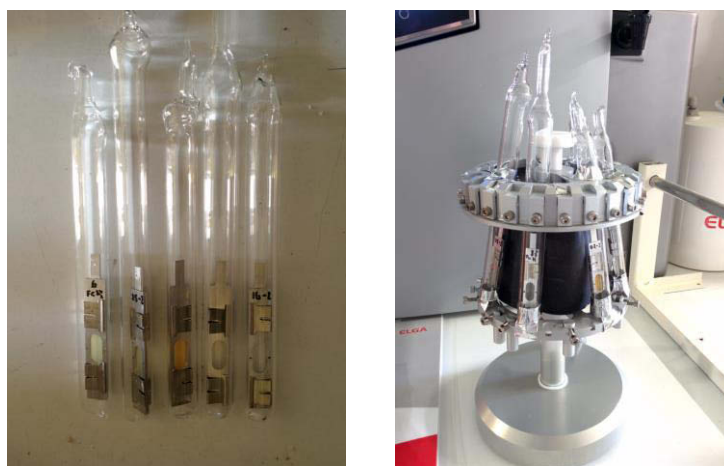
Figure 76 Photographs of organic composite films in vacuum-sealed glass tubes.
