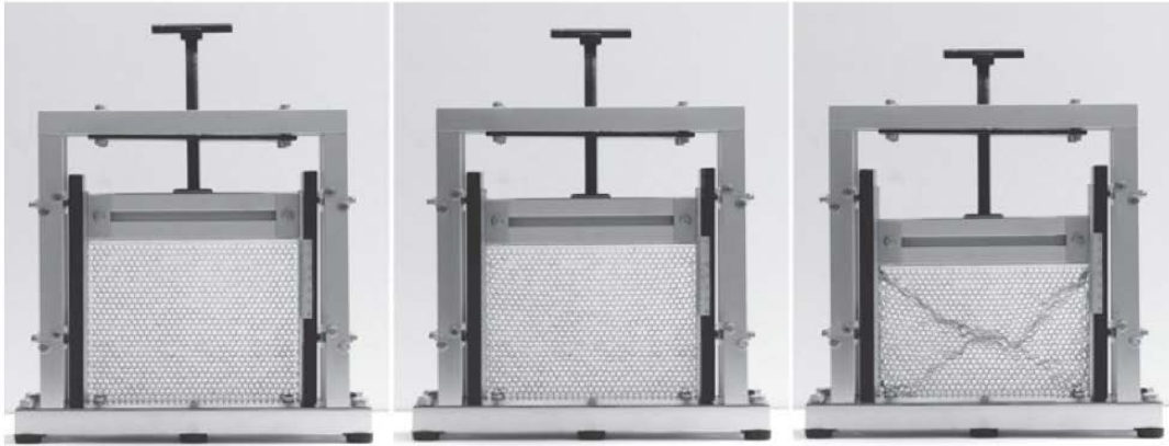
Figure 5.1: Experiment performed by Poirier et al. [90] (image taken from [12]) on a 2D regular array of hollow soft cylinders confined in a rectangular box. The compressive loading is applied via the piston. Note the localization of the deformations on the last image.
