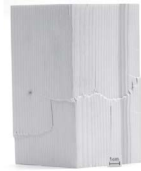
Figure 1.2: Fracture due to deformation localization on a prismatic spruce wood sample compressed in parallel to the fibers. Image reproduced from [12].
